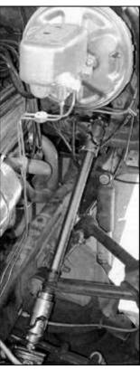
25...Once you've got the box connected to the steering column, fill the system up with fluid. With a dry box, you'll want to fill the reservoir up and then turn the engine on to cycle fluid through the box. This may take a few times, but make sure to get it filled properly to avoid any damage. From there, hit the road and enjoy your rehabilitated steering.
