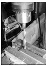
23...Then drill the shaft, but only through one side, as you want the set screw to bottom out against the other side's inner wall.
