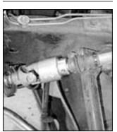
20...The same goes for the lower application. On the steering box's 13/16-36 output shaft, you'll notice the splines are separated by a recessed groove-make sure the U-joint slips over that, allowing the set screw to lock fully.
