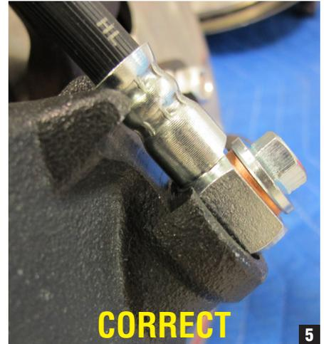
5. Properly installed and tightened, no portion of the brake hose fitting (other than the copper washer) should come in contact with the caliper body, as shown. (photo 5)
