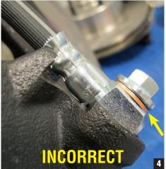
4. Installed backwards, as shown, the shoulder of the hose fitting will come in contact with the caliper, causing the banjo to crush the compression washer at an angle, ultimately leading to fluid leaks. (photo 4)
