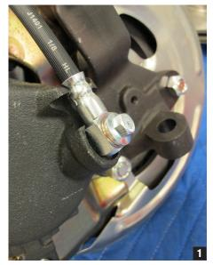
Banjo-style rubber brake hoses with an offset fitting must be installed with the notched side facing outward in order to attain a complete, proper seal. (photo 1)
