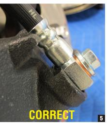
5. Properly installed and tightened, no portion of the brake hose fitting (other than the copper washer) should come in contact with the caliper body, as shown. (photo 5)
