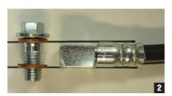
The reference marks indicate "top" and "bottom" of the banjo fitting; the stepped side (top) faces outward, allowing the bottom to seal tight onto the caliper without coming in contact with the fitting's crimped shoulder. (photo 2)
