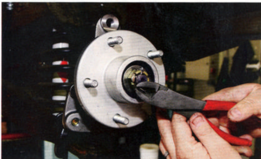
When sliding on the washer and castle nut, we tightened the castle with a wrench to seat the bearings. Then we backed the nut off, finger-tightened it to take out the slack, and inserted the cotter pin. Never tighten the nut down on the bearing with a wrench and leave it that way; too much load can cause premature bearing failure and potential spindle damage.
