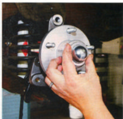
A couple taps from the rubber mallet is all you need to seat the dust cap in place, and the hub is as good as done.
