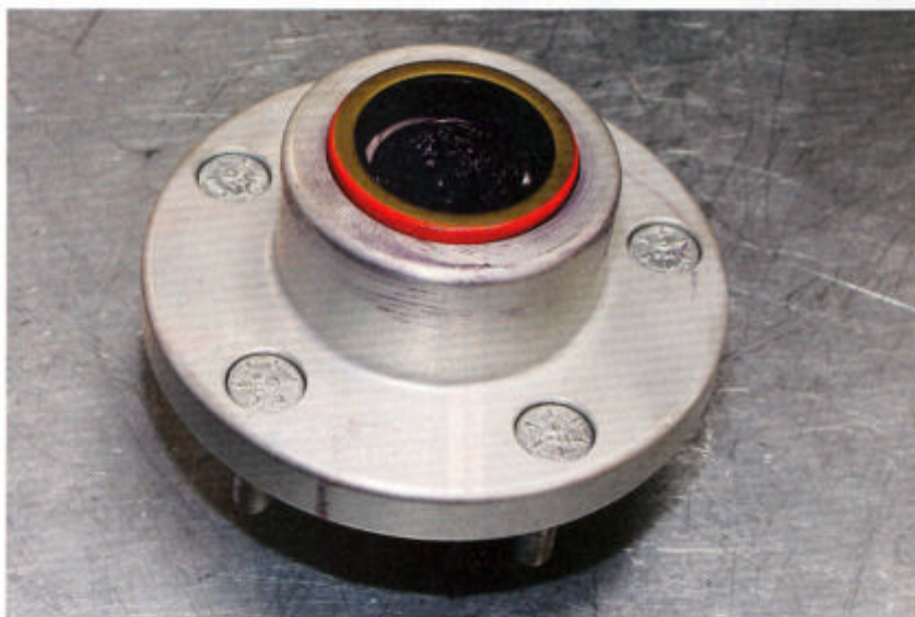
Lastly, the new seal is tapped into place, keeping it all together.
