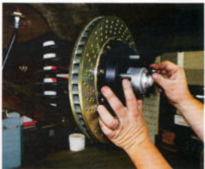
Here is the beauty of these two-piece 13-inch rotors. The rotors are built in such a way that they're considered floating rotors. Every other disc mounting screw has approximately 0.001 inch of play and is held in place with a spring bushing. The spring keeps constant tension on the bushing and fastener, eliminating rattles or squeaks from road vibration. The two-piece hat and rotor system has distinct advantages over a one-piece, including weight savings; nearly 8 pounds is saved on each front corner of the vehicle. Additionally, the direction vanes and cross-drilling help to further dissipate heat. These two features result in more consistent braking and heat dissipation of the rotor.
