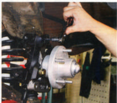
The aircraft-grade precision-machined aluminum bracket which holds the caliper in place attaches to the spindle as shown here. What sets the Brembo fixed brakes apart from other fixed calipers is the radial-mounted fixed caliper. All Brembo brakes are radial-mounted and no shimming is required to set the caliper's position, resulting in longer pad life and far superior braking.
