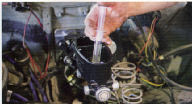
28 Bleeding the brakes started with the Wilwood master cylinder and then worked from the farthest point forward. A Wilwood proportioning valve was installed under the hood.
