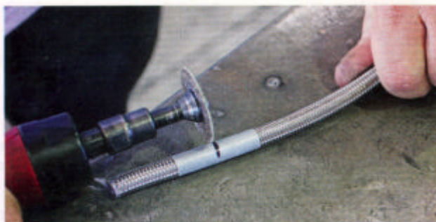
25 The CPP Hydratech uses hydraulic force generated by the power steering pump. A die-grinder with an abrasive disc was used to cut the braided stainless steel line to length. Note the duct tape used to prevent fraying.
