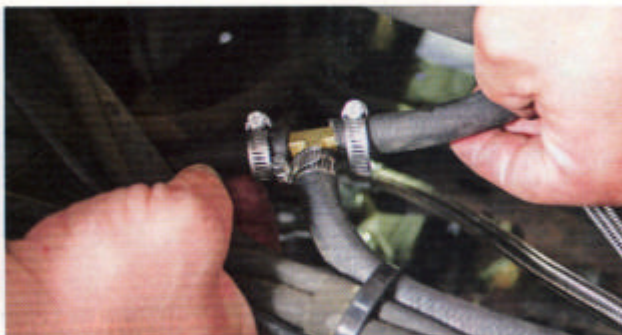
27 The routing specified for the hydraulic lines at the T-fitting defies aesthetics, but a big loop must be used to ensure proper hydraulic flow.
