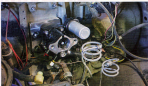
23 The CPP Hydratech hydraulic brake booster's billet aluminum flange mounts with four easy-to-reach bolts to four existing holes.
