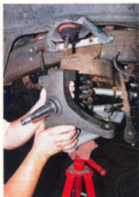
15 Here the CPP modular spindle is being inserted into the upper and lower ball joints. Notice the truck has already been equipped with CPP tubular control arms.
