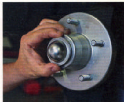
18 Next, Craig installed the dust (grease) cap by using a piece of pipe that matched the diameter of the cap's outer lip.
