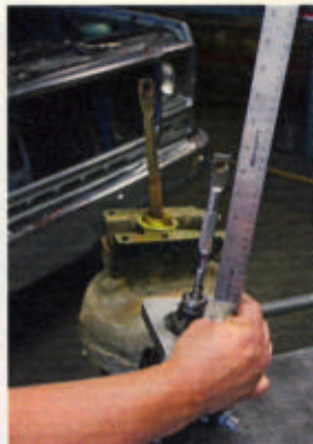
22 An important step, before mounting the CPP hydraulic brake booster, Craig measured the stock travel (push) rod's length to match it to the new CPP booster.
