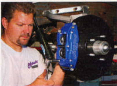
19 With the 14-inch front brake rotor mounted onto the hub, the Wilwood modular caliper mount was then positioned into place and the Wilwood 6-piston caliper tightened down on top.
