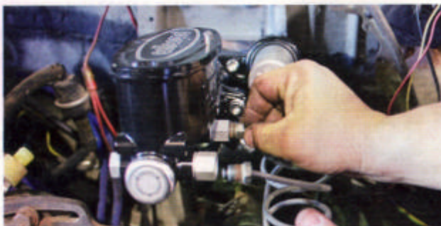
24 Next, the high-capacity Wilwood dual master cylinder was bolted up to the CPP Hydratech. Then using fitting adapters, included in the kit, the stock brake hydraulic lines threaded right up without bending the lines.
