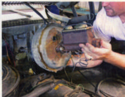
21 The stock dual master-cylinder with a vacuum brake booster was removed by unbolting its six mounting bolts of which two are a real bear to get to.
