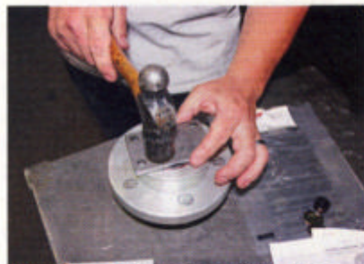
17 After packing the tapered wheel bearings with premium grade wheel bearing grease intended for disc brakes, Craig installed the hub grease seal, flush against the hub.
