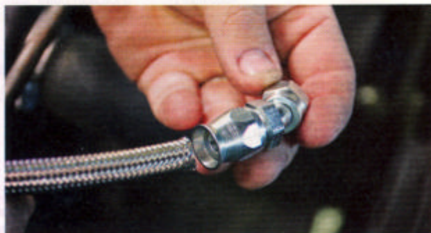
26 After the CPP Hydratech's hydraulic lines were cut to length and the fittings attached, the power steering (pump) system was flushed and then topped-off with Amsoil synthetic power steering fluid.
