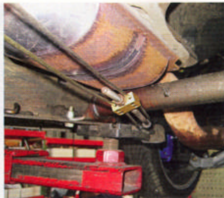
30 This is how the rear section of the e-brake linkage appeared after it was connected. The next phase will be in an upcoming issue where we get the '79 back out to the track and see what kind of braking numbers the monster 14 1/13-inch Wilwood 4-wheel disc brake combination delivers.
