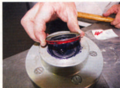
16 The Wilwood kit includes a billet hub manufactured by CPP at their Anaheim, California, location. The CPP hub utilizes the larger Timken style wheel bearings found on trucks (not all hubs do).
