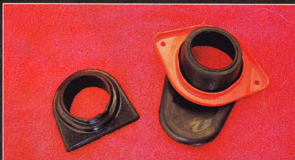
Before we install the new column it's necessary to inspect and replace a few components as necessary. For these, we went to one of the largest reproduction parts houses in the world, LMC Truck. The seals at the top and bottom of the stock column were thrashed, so we decided to play it safe and ordered not only the floor and upper seal, but the lower seal retainer as well.
