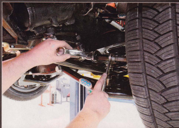
Once in place, the billet adjusters are locked down using the lock nut at either end.
