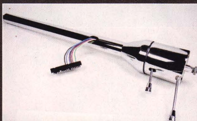
Here's a beautiful chrome version of the same Retrofit Series tilt column we're using from ididit. These columns feature an eight-position tilt, stock GM-style 3/4-inch wiring harness, 3/4-36 output spline, four-way flashers, self-canceling turn signals, knobs and handles, and are compatible to stock GM steering wheels as well as a number of three-, five-, six-, and nine-bolt steering wheels via an adapter.
