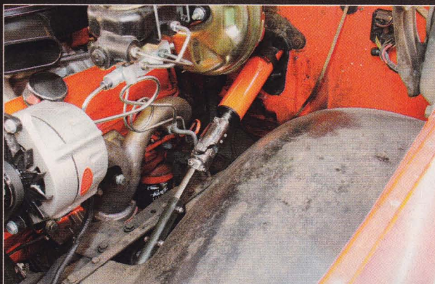
Here's the final assembly of the steering shaft, from column to rag joint sleeve.
