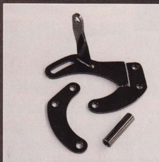
Mounting the engine accessories created a slight problem as the early heads were not drilled out to accept any brackets. Alan Grove Components solved this problem for us by providing a set of brackets and pulleys to ensure all the accessories will line up nicely, including the power steering pump.
