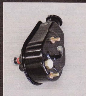
Mounting the engine accessories created a slight problem as the early heads were not drilled out to accept any brackets. Alan Grove Components solved this problem for us by providing a set of brackets and pulleys to ensure all the accessories will line up nicely, including the power steering pump.
