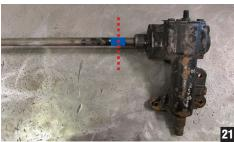
Now you can cut the inner steering shaft off the stock steering box. From the base of the steering box measure up 2" and use blue painters tape again to make a square mark. It is also important to cut this shaft off square as well. (photo 21) Measure 2" up from the bottom of the steering shaft you just cut and mark the shaft. Using the supplied rag joint (#RJC-605X) grind or machine two flat spots into the steering shaft the full 2".
