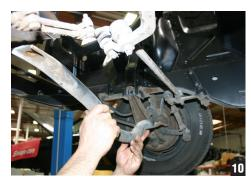
With the steering linkage and pitman arm loose it's now recommended to take the stock crossmember off temporarily to allow the steering box to be removed as one piece. This crossmember is bolted to each side of the frame so remove the hardware on each side and pull the crossmember out. This is reinstalled once the steering box is out of the car. (photo 10)
