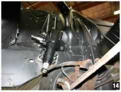
Now you can hang the new gearbox in place on the subframe. The gold bracket bolts to the hardware coming though the subframe from the previous step. The socket Allen head bolts hold the steering box to the gold bracket. With the box tightened up the input shaft should be aligned dead center to the opening in the firewall where the column comes though. (photo 14)
