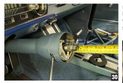
Once the rag joint and the roll pin are securely fastened to the gear box, double check one last time that the steering shaft is in the correct position for steering wheel to column positioning. (photo 30)
