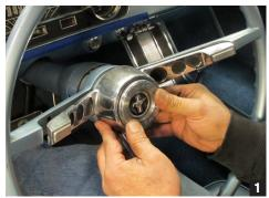
Start by removing the stock horn button. The horn button is simply pushed in and rotated counterclockwise. This will allow access to the horn contact spring and steering wheel nut. (photo 1)
