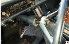
With the turn signal switch, spacers and spring re-installed you can now put the steering wheel back in place. Confirm the steering box and wheels are straight and centered and mount the steering wheel back in center. (photo 32)
