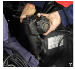
From the wheel well position remove the stock mounting bolts to the steering box. Make sure to hold the gear box when removing the last bolt so you don't drop it out as the inner steering shaft inside the car could cause damage to the dash. Once loose carefully lower the steering box out of the engine bay down from the bottom of the car. (photo 11)
