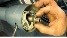
There is a small cone shaped bushing used to center the column tube from the factory. This needs to be pulled out to allow the outer column tube to be removed from the car. This part is also used again for reassembly. (photo 7)
