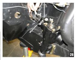
Once you confirm your upper measurement now is time to mark and drill the roll pin hole. If you can accomplish this while in the car you can simply drill the hole. If you have limited space simply remove the inner shaft again and drill it out with a drill press. (photo 28)
