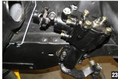
Install the rag joint onto the steering box. Remove the Allen head bolt from the rag joint and slide it onto the shaft; when the opening is visible though the hole in the rag joint put the Allen bolt back through and tighten it up. Make sure it is tight enough to remove any slop. (photo 23)
