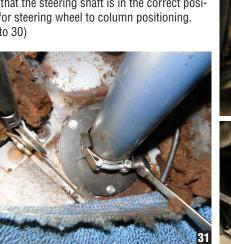
The attaching ring now gets bolted in place and the clamp will secure the column tube to the bracket. Do not over tighten this assembly. It is OK to just snug this to keep it in position. (photo 31)
