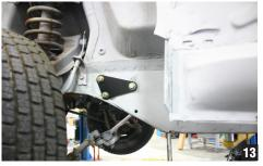
The new steering box has a special triangular mounting plate that is installed on the wheel well side of the subframe with the mounting bolts going though into the engine bay. Make sure this plate is installed here and not on the engine bay side. (photo 13) Confirm that your gearbox is centered by moving the input shaft all the way to the internal stop (right or left) and count the amount of rotations and bring the gear box back to center. Then install
