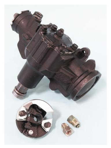
The #CP7525 is a direct bolt-in for all 1964-95 Saginaw 605/800-Series equipped GM full-size passenger cars, as well as various other non-GM makes/models. However, depending on year and model, input shaft and line fitting types may vary.
