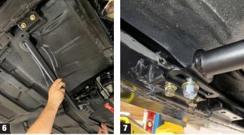
Install crossmember onto adjustable brackets; leave carriage bolts loose. (photos 6 & 7)
