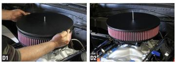
Test fit the air cleaner assembly (not included) onto the air cleaner stud to verify correct stud height (Fig. D1-D2). If needed, the air cleaner stud must be removed and cut to allow proper fitment of your specific air cleaner height or for hood clearance. (Fig. E1-E3)
