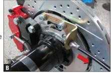
3. Identify the mounting locations necessary for your install where the cable housings will end. For most configurations, an original parking brake cable mounting tab will be used. Install the cable adjuster bulkhead fittings into the mounting tabs so they are threaded a neutral distance (about half to three-quarters of the way) through the tabs. This will allow for future cable length adjustment if needed. (FIG. D)
