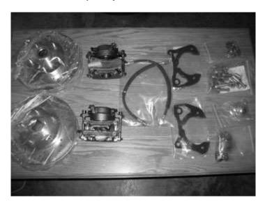
This page describes the installation of Classic Performance Products' 64-67 stock spindle front disc brake conversion kit, and the MCPV-1 master cylinder.
