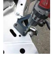
2. Using the empty rivet holes loosely attach the new engine mounts to the cross member. You will need to install two bolts into each mount through the slotted holes in the new mounts and into the frame: the nuts will be installed on the inside of the front crossmember.
