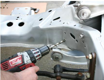
1. Remove the four rivets on the rear face of the front crossmember. There are two rivets per side, these connect the sides of the frame with the crossmember.
