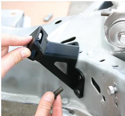
4. Using the new mounts as a guide drill four holes 3/8" through the top of the crossmember. Install the remaining bolts through these new holes, again the nuts will be on the inside of the crossmember.
