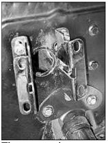
These mounting brackets tilt the booster slightly, which changes the pedal ratio in order to get a full stroke out of the master cylinder.
