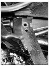
As per the directions, Alan drilled a new hole in the pedal arm 1 inch lower than the original. The reason for this is that it makes the pedal less "touchy."
