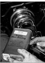
CPP even carries topof-the-line brake fluid, which we then used to fill the master cylinder reservoir.
