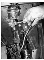
We soaked most of the brake fluid out of the reservoir with a rag, and then detached the old brake line with a line wrench.
