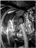
We then ran the vacuum line over to the fitting on the booster.
