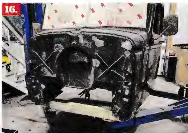
15-17. In tidying up the engine bay, the frontend sheetmetal was removed to begin the task of weld-filling a myriad of unneeded holes on the firewall with sheetmetal to give it fresh look. The area was then sprayed with epoxy primer and finished with SEM Hot Rod Black.
