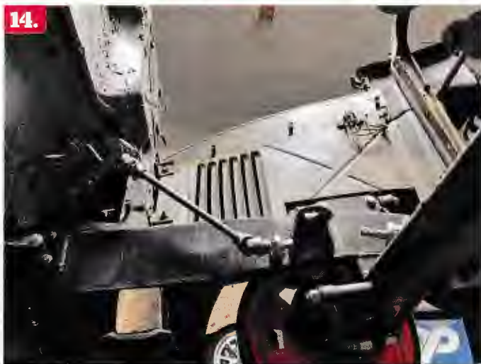
12. With the truck now a roller, in the care of Pat O'Brien at Precision Industries, it was time to mock up the engine and transmission mounts for the driveline.
