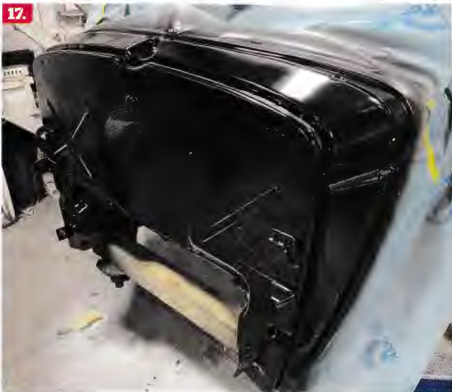
15-17. In tidying up the engine bay, the frontend sheetmetal was removed to begin the task of weld-filling a myriad of unneeded holes on the firewall with sheetmetal to give it fresh look. The area was then sprayed with epoxy primer and finished with SEM Hot Rod Black.
