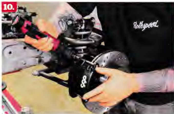
10. The freshly powdercoated black calipers came with the pads already loaded into the assemblies, making installation a snap. The completed front and rear disc brakes look great and will add plenty of newfound stopping power to the truck.
