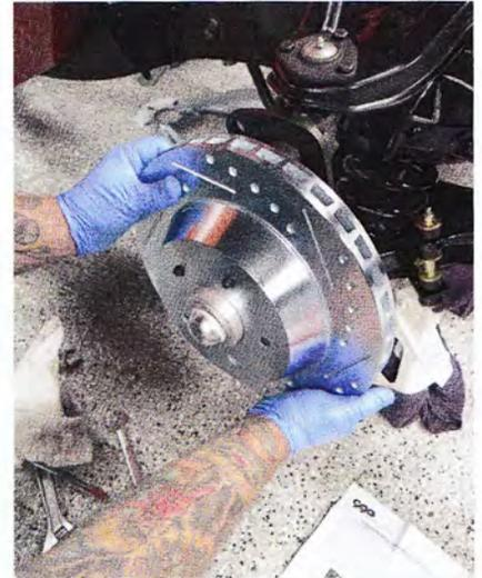
**7** Install the new rotors on the hubs. Hold the rotor in place with a couple of lug nuts.
