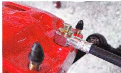
**12** Install the new brake hoses on the calipers with the new crush washers (one on each side of the hose fitting) and new brake hose bolt. Install the other end to the brake lines. Tighten with the 11mm flare nut wrench.
