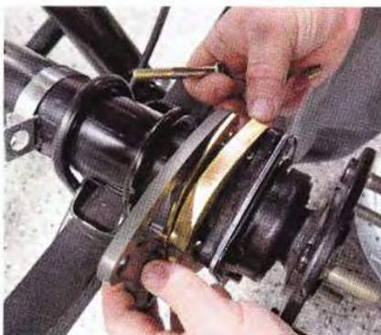
**20** The shim(s) will go between the two caliper bracket halves; the bolts must be completely removed in order to install them.
