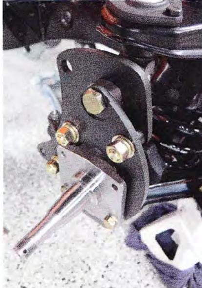
**3** Install the caliper mounting portion of the bracket. It requires three spacers between it and the main bracket, with the bolts installing from the rear. The boomerang-shaped bracket will angle down, toward the rear
