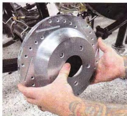
**18** Install the rotors onto the axles; hold in place with lug nuts. As with the front, the rotors are marked (L/R) for orientation.
