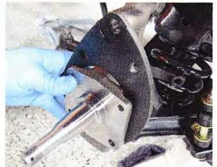
**1** Start at the front by installing the new two-piece brake caliper brackets on the spindle. If replacing spindles, you will need to do so now—a spring compressor will be necessary to safely perform this step. The main bracket mounts on the wheel side of the spindle on the top, and between the spindle and the steering arm at the bottom in the rear.
