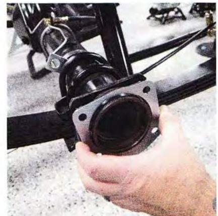
**15** Install the bearing spacer (simulates backing plate) onto the axle housing with the flat side facing upwards.
