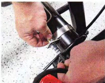
**22** Install the brake hose tabs and clips onto the new brake hoses. Connect the brake hoses to the hard lines. You may need to modify the hard lines to get a proper or clean fit. Secure the brake hose tabs around the axle with the tab clamp. When everything is in place, using your 10mm flare nut wrench, tighten the ends starting with the hard line. Tighten the bolt against the crush washers in the caliper.
