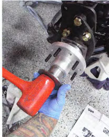
**6** Install the grease cap by tapping in with regular hammer and socket, or a rubber mallet and steel tubing, as we did.
