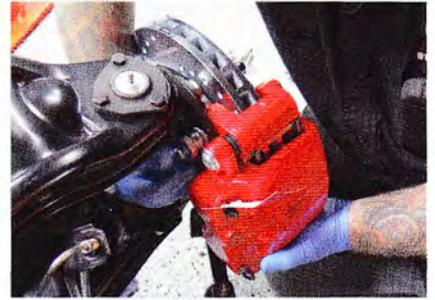
**9** Install the calipers on the caliper mounting brackets. The calipers install with the bleeder pointing upward or you will not be able to properly bleed the brakes. The caliper ear goes between the rotor and the bracket and mounts with the two caliper mounting bolts, flat and lock washers that are provided in the kit.
