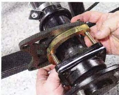
**17** The two-piece caliper brackets will install on the inside of the axle flange on the rear end housing, with the bolts inserting from the rear towards the rotors. From here, you will need to determine whether or not caliper shims are required.
