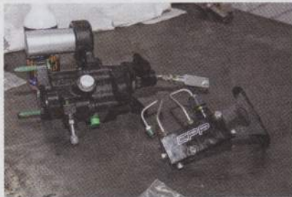
12. Here's how the CPP proportioning valve and Street Beast booster should appear after separating.
