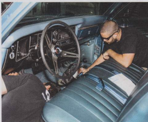
5. In order to disconnect the master cylinder, the brake master cylinder pushrod was disconnected inside the firewall by removing the clevis pin retainer clip on the brake pedal.
