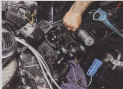
13. The Street Beast booster must be installed to the firewall minus the master cylinder.
