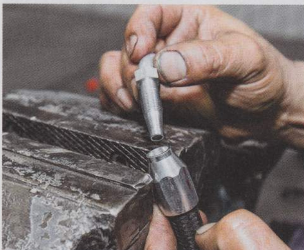
24. Next, the male portion of the fitting is screwed in and tightened down. As a precaution, it's always a good idea to install a CPP inline filter into the Street Beast's feed line.
