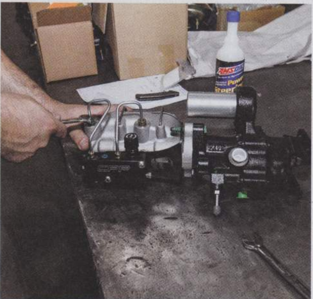
11. Bench bleeding the master cylinder to ensure there are no air bubbles in the system is an absolute must. Prior to bleeding, the CPP master cylinder must be removed from the proportioning valve and Street Beast booster.
