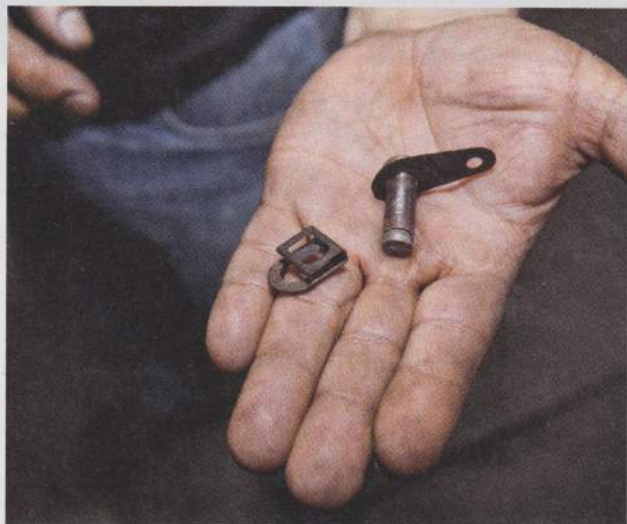
6. A real bear to disconnect; this is what the stock clevis pin and retainer clip look like. The eyelet is for a return spring to attach to.
