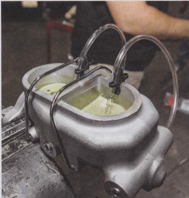
18. In order to bench bleed the master cylinder it must be clamped securely into a vice. Next, the bleeder hose fittings with hoses must be screwed into the output ports. Note how the hose clips hold the bleeder hoses in place. Fresh brake fluid was used to fill both reservoirs.
