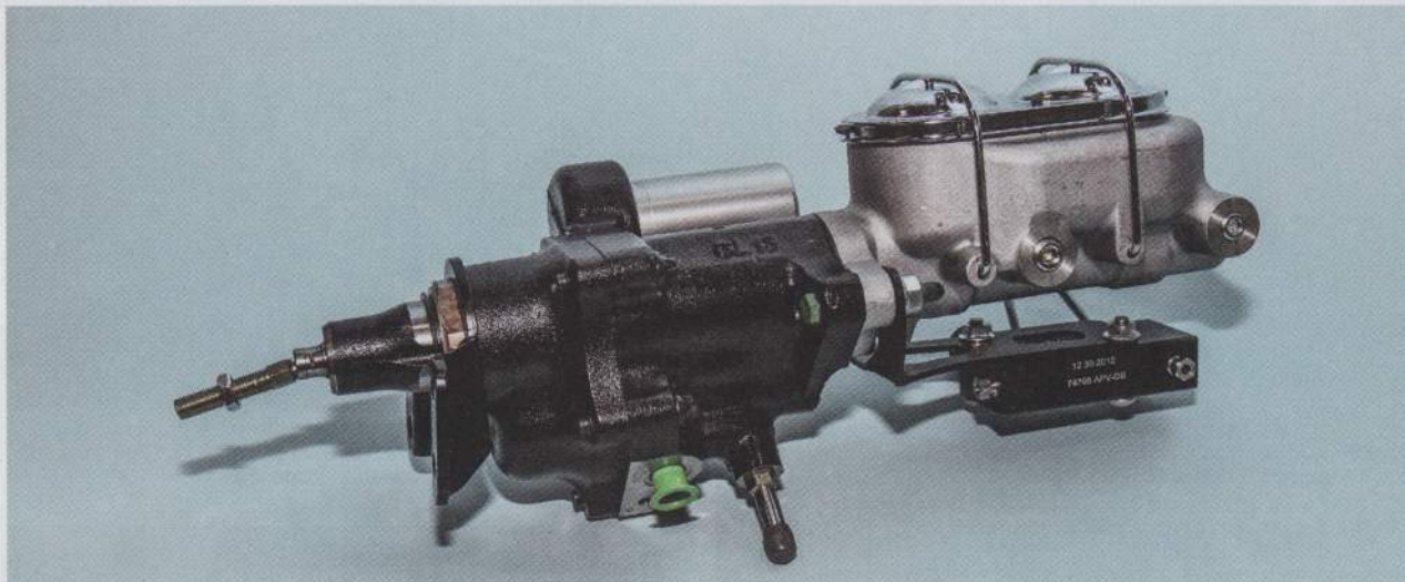
1. Classic Performance Products' Street Beast is a compact, well thought out unit. Notice it comes equipped with an adjustable proportioning valve mounted in close proximity to CPP's proprietary Corvette-style aluminum alloy master cylinder.
