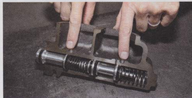
17. Front-to-front brakes and rear-to-rear brakes: This cutaway master cylinder reveals how both chambers (pistons) operate in tandem simultaneously to pressurize the front and rear brakes.
