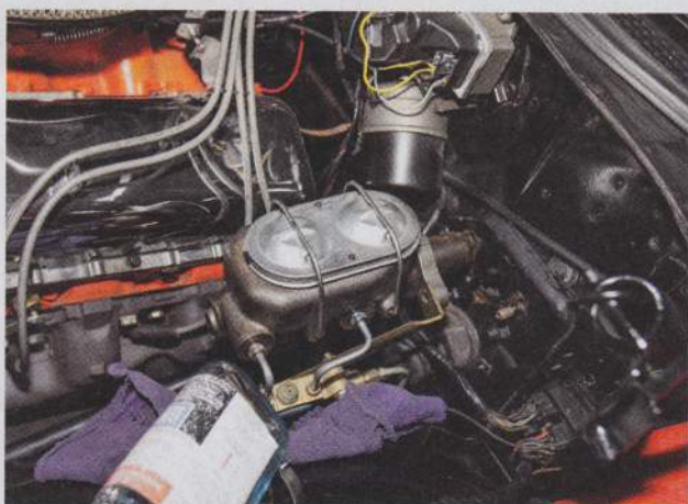
9. Care should be taken not to kink or bend the steel brake lines connected to the master cylinder as it is pulled forward off the studs. Slight forward bending of the steel tubes is allowable if done with care.
