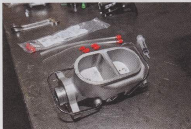
16. This photo illustrates how completely the master cylinder must be disassembled in order to be bled properly. Notice the CPP brake bleeder kit (included) behind.
