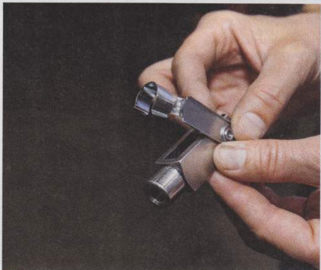
7. This much easier to install clevis is included with the Street Beast's installation kit.
