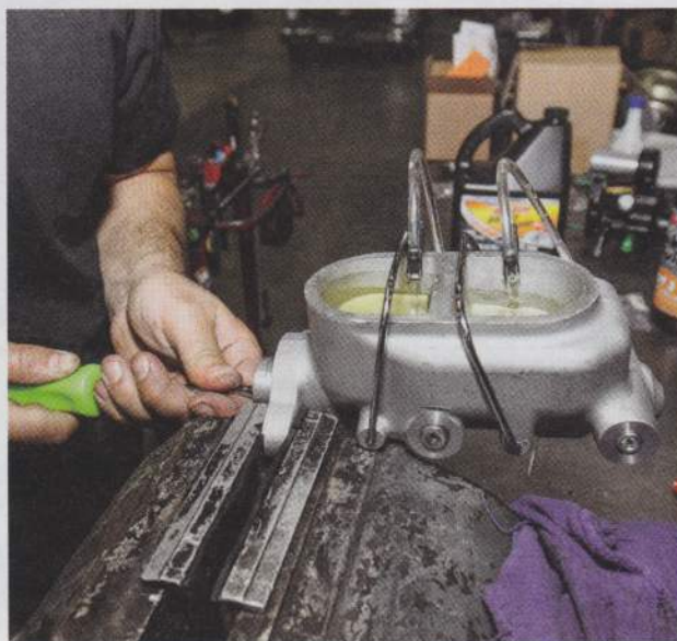
19. A round Phillips screwdriver was used as a pushrod to pump the master cylinder. Notice the air bubbles escaping from the two hoses as the master cylinder is pumped.
