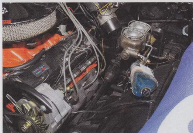
3. To supply the Street Beast with operating pressure, the vehicle must be equipped with power steering. CPP offers power steering conversion kits for cars without power steering. Note Frank's El Camino lacked power brakes and had an improperly sized master cylinder that contributed to ineffective braking.
