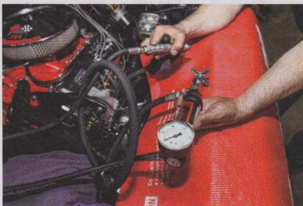
4. Never skip this vital first step: Before installing the Street Beast, the existing power steering pump had to be tested to ensure its output pressure was up to specification.
