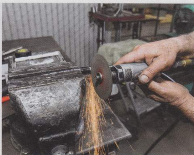
23. A 4-inch cutoff wheel on a die grinder is the best method to cut the hose, leaving a minimum amount of ridge (flare), allowing the female portion of the fitting to fit snugly.
