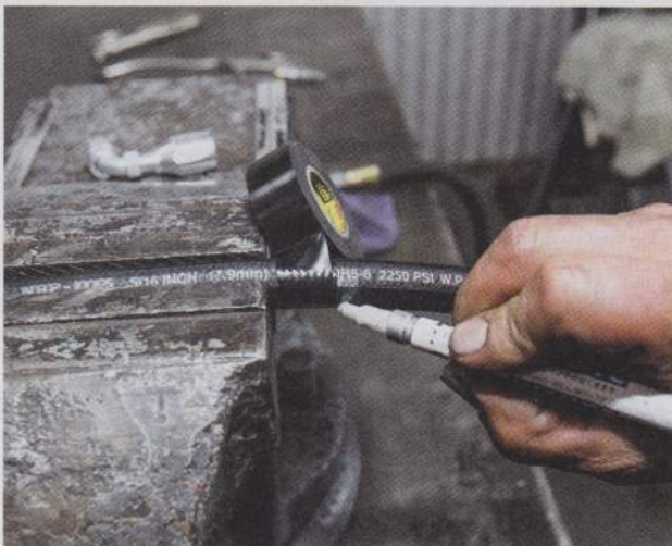
22. After determining the right length of hose to plumb the Street Beast with, the fittings can be installed. Wrapping the hose in electrical tape works best to indicate where to cut the hose.
