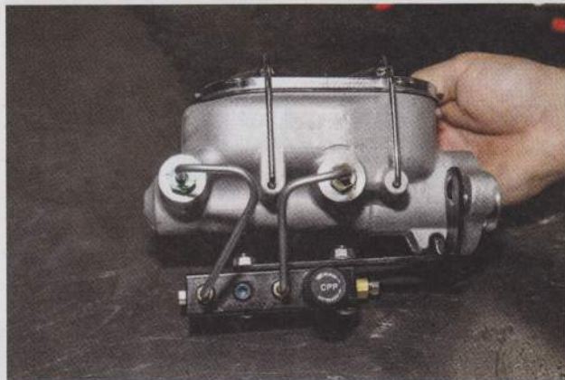
15. To adjust the CPP self-contained proportioning valve, the adjustment knob is turned clockwise to increase pressure and counterclockwise to decrease pressure.
