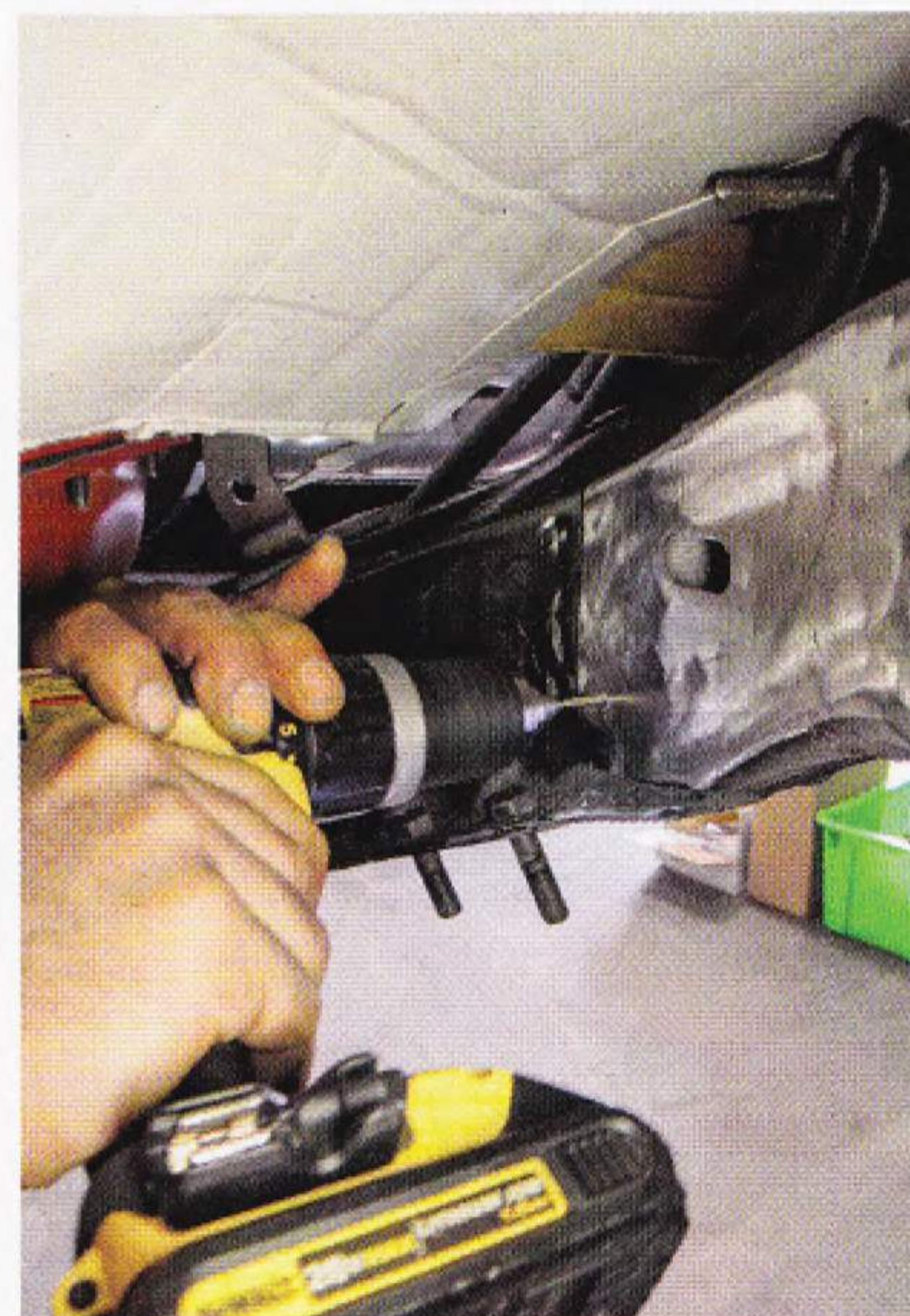
05 With the mounts out and the crossmember rivet heads ground flush with the framerrail, the bodies of the rivets are drilled (3/8-inch bit) and subsequently punched out.
