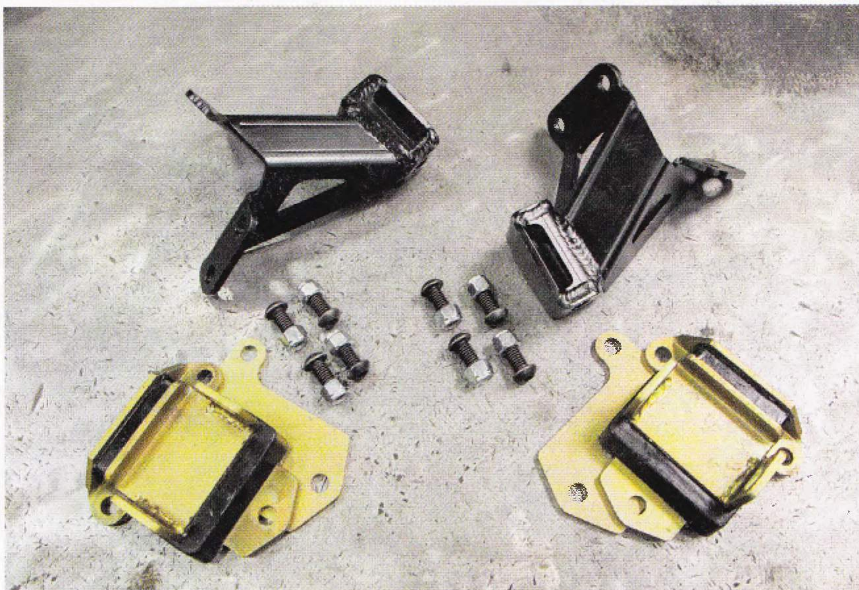
01 Fabricated out of 3/16-inch steel plate, CPP's 1955-'57 Chevy pedestals locate a small-block V-8 3/4-inch forward (also available in stock location) and utilize standard rubber or upgraded poly engine mounts.
