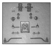
In addition to the trick spindle swap, we decided to step up and replace our worn components with these fresh pieces. Fresh ball joints, hardware, tie rods, bushings, and shock tower brackets will help us sleep at night, and hard launches at the strip won't be as scary.
