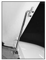
Two more holes were measured and drilled into the bottom edge of the hood as per the directions. Then a machined block was bolted into place for the prop rod to plug into.
