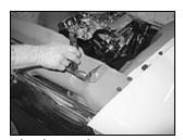
The lower hinges were bolted to the grille support using an existing hole. By installing the pivot bar (this time permanently and with a dab of grease), we could determine exactly where the second hole for the bracket needed to be drilled and bolted.
