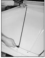
The stock support rods were removed from the rear of the hood. You can then use them to pry on the front two brackets to expose the three welds that hold each of them on.
