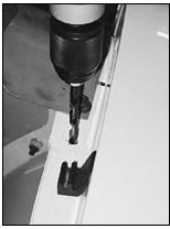
All that was left to be installed was the polished stainless prop rod. A hole was measured out and drilled into the fender edge between two mounting bolts.
