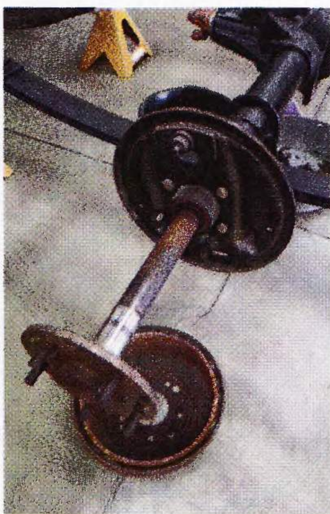
04 Disassemble the drum brake mechanism (including brake lines/e-brake cables, if applicable) and remove the axles—inspect the bearing surfaces on the axle shafts for excess wear/pitting as well as the condition of the bearings themselves; replace if necessary.
