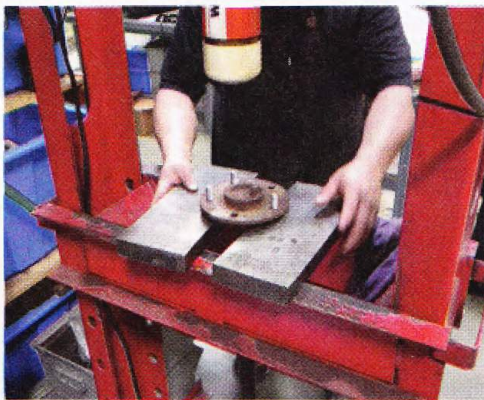
07 Using a hydraulic press (or have a machine shop perform the work), squarely press the new wheel studs in.
