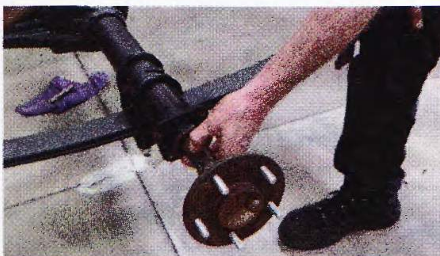
08 With the new studs completely pressed in, the axles can be replaced in the rearend—and the C-clips reinstalled to secure the side gears during the remainder of the brake kit upgrade (you can wait till everything's finished up before sealing and attaching the differential cover).
