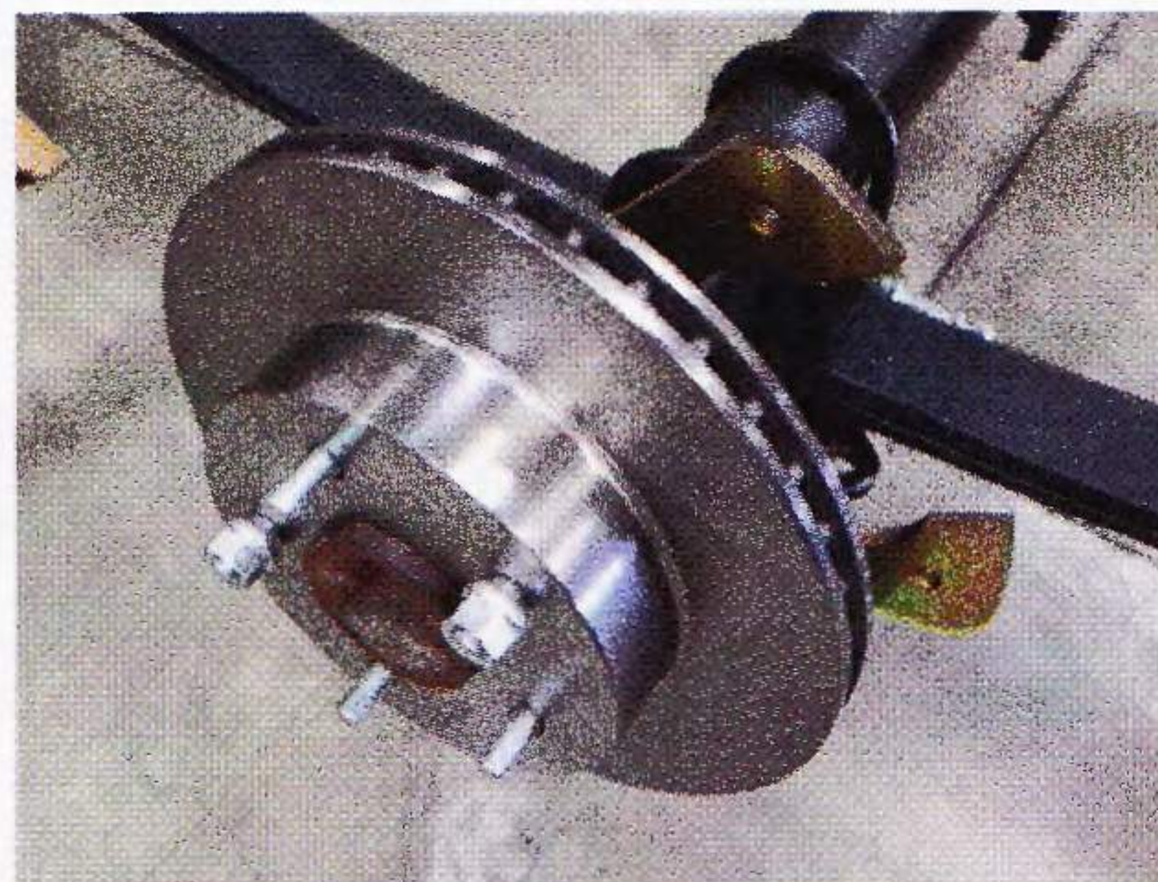
11 Hang the rotor on the axle, holding it in place with a couple lug nuts. Make sure the register of the rotor fits flush (no burs interfering) onto the axle.
