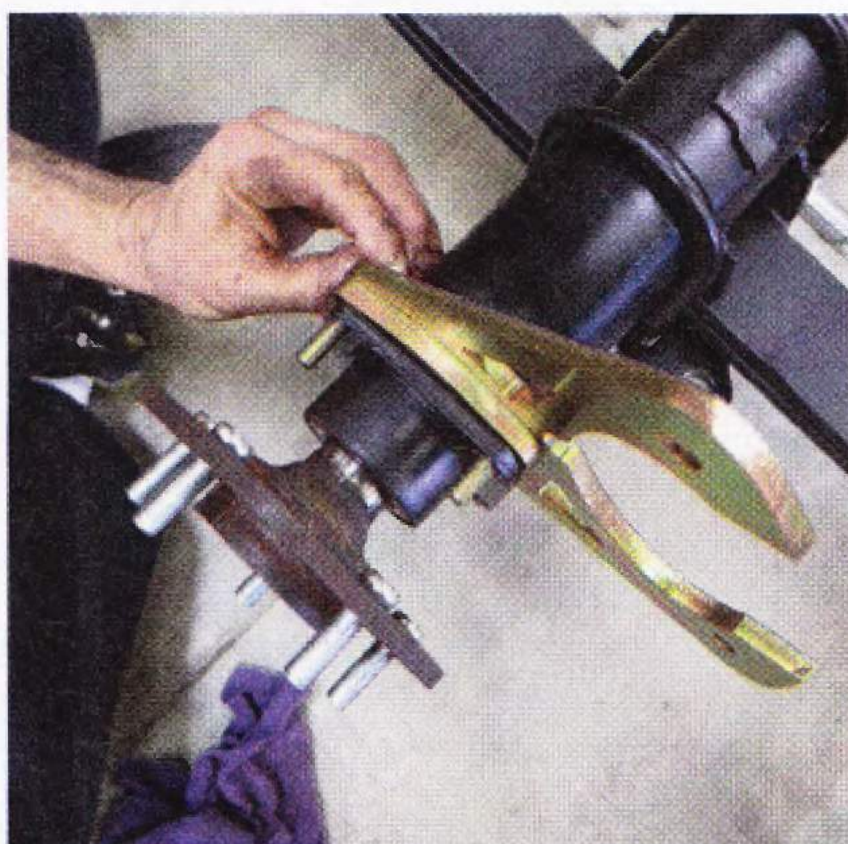
08 With the new studs completely pressed in, the axles can be replaced in the rearend—and the C-clips reinstalled to secure the side gears during the remainder of the brake kit upgrade (you can wait till everything's finished up before sealing and attaching the differential cover).
