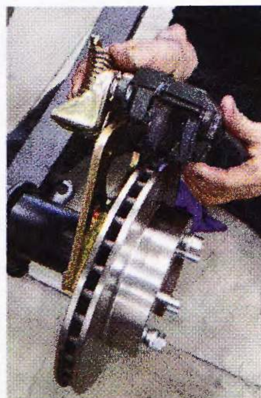
12 With the slide pin bushings pressed all the way toward the back side of the caliper (making sure they move freely), install caliper into the bracket. In some cases, as illustrated here, the offset of the bracket may place the caliper too far
