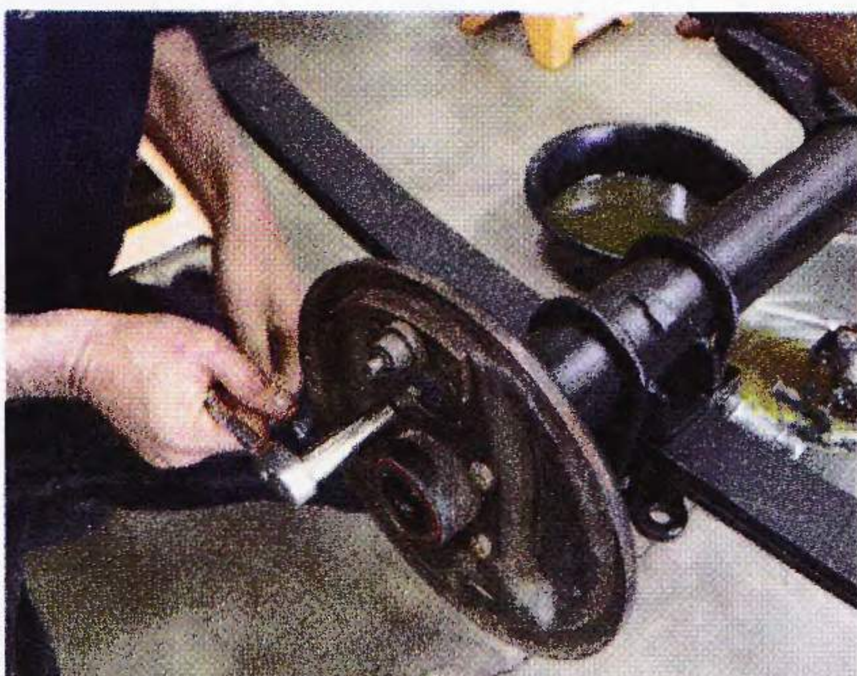
05 Remove the backing plates from the rearend housing.
