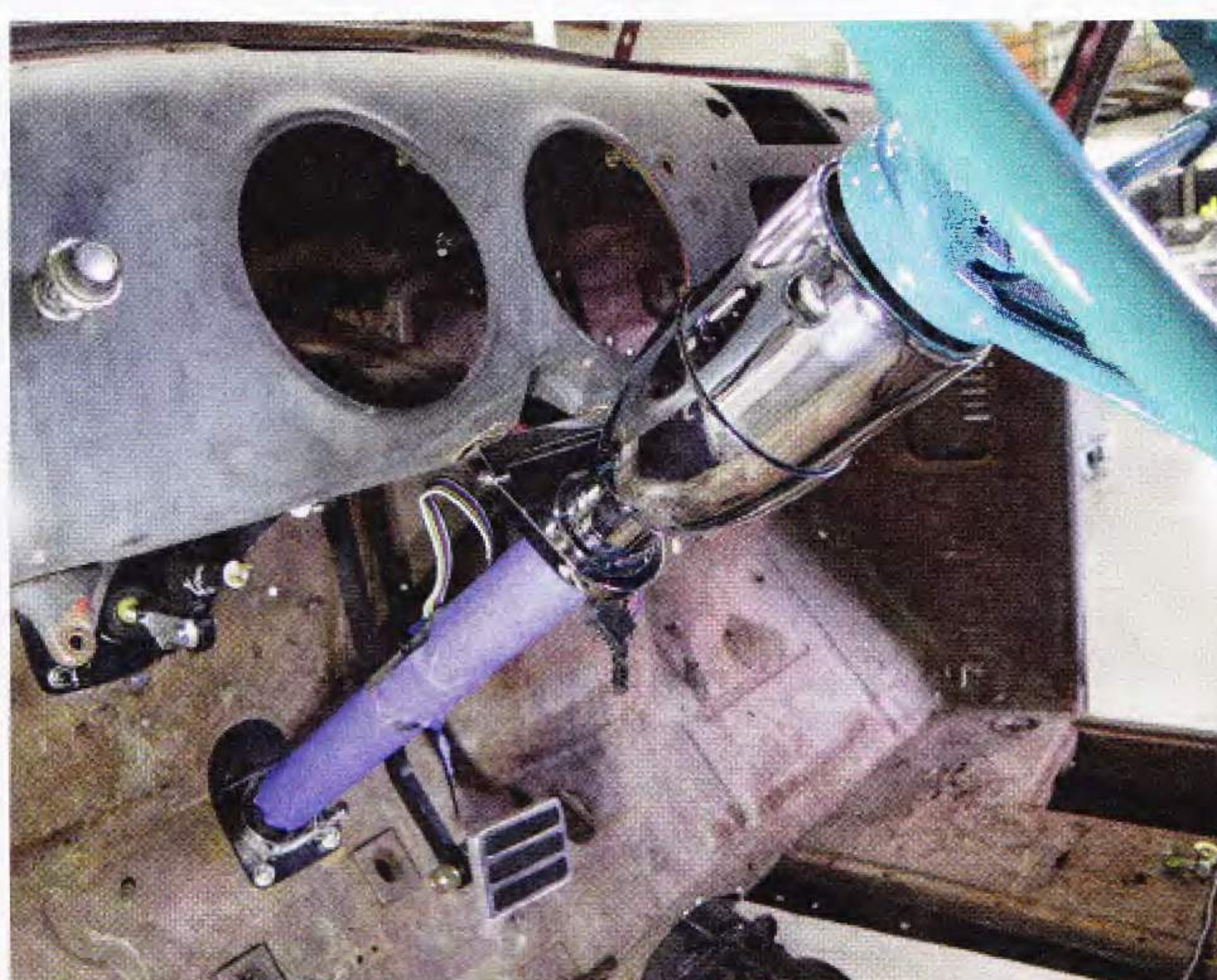
17 ... we installed a new CPP tilt column to ensure a complete package fit. Stay tuned for the full steering component installation!
