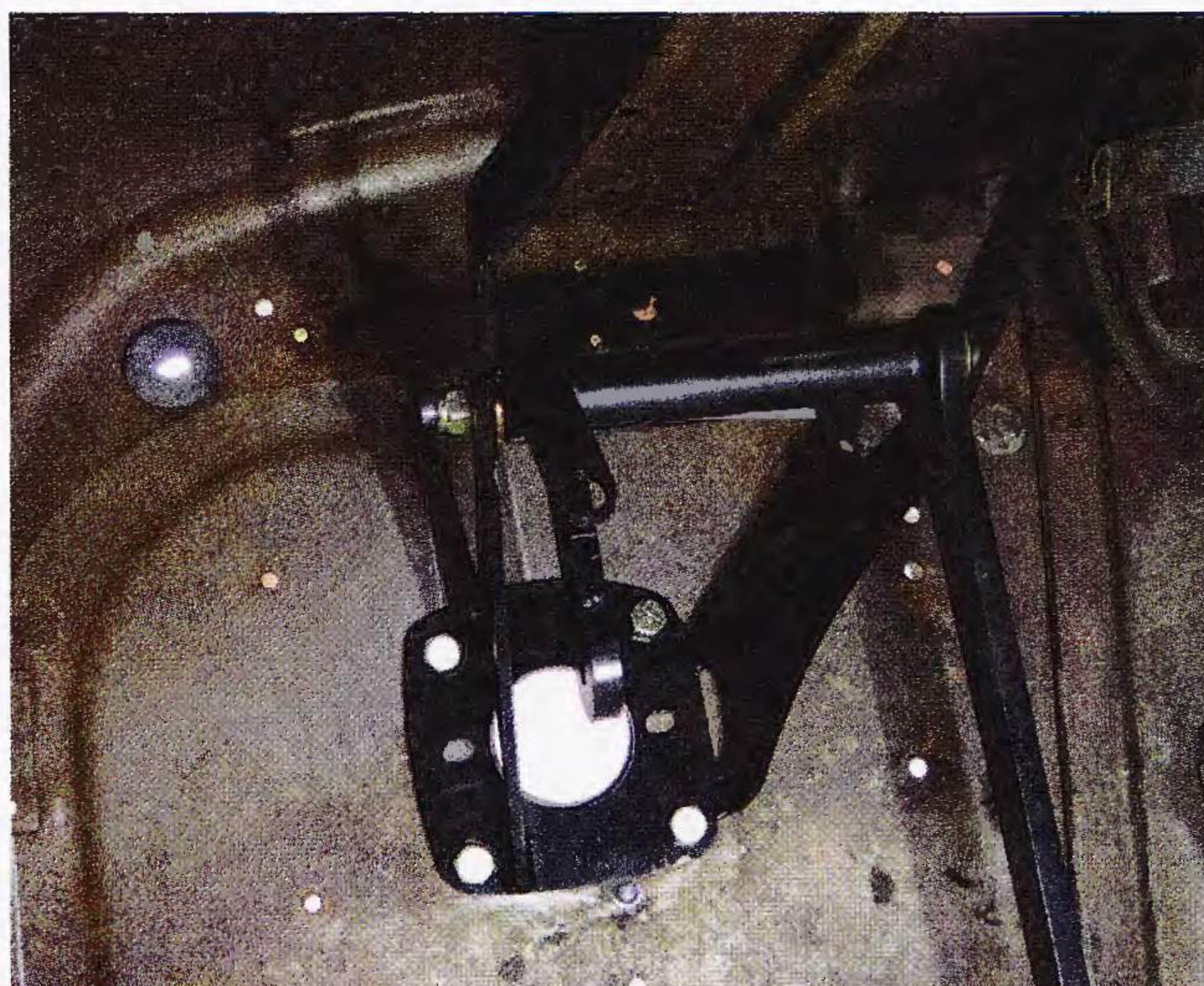
12 The bracket is temporarily bolted back onto the firewall to verify hole placement (just in case) and any sharp edges are deburred.
