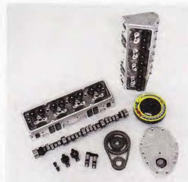
**03** To enhance performance we selected aluminum heads from RHS, a COMP retrofit roller hydraulic cam and kit, and a TCI Rattler crank damper.
