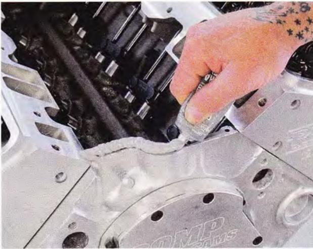
**21** Rather than use intake manifold end seals (which tend to squeeze out) a bead of silicone was applied to the block's bulkheads.
