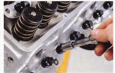
**14** Head bolts, as well as all the other engine fasteners, are from ARP. Note the washers used with aluminum heads.
