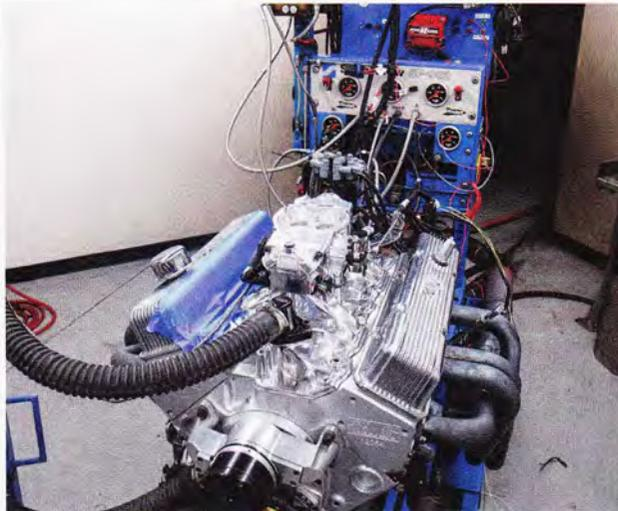
**26** Strapped to the dyno at Westech, our 350 used an MSD ready-to-run distributor and a Holley Terminator EFI system.
