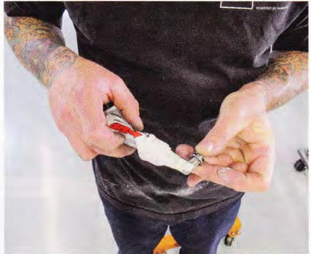
**22** Antiseize was used on all the ARP stainless fasteners to prevent galling of the threads.
