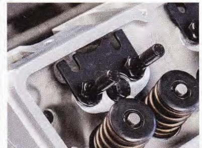
**15** The RHS heads came with 2.02-inch intake valves, 1.60 exhausts, screw-in studs, and pushrod guideplates.
