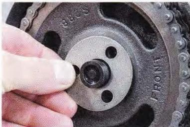
**09** With the shim in place the bearing was reinstalled and secured with the retainer plate. Rearward movement is limited by the cam sprocket pressing against the block (as with flat-tappet cams).
