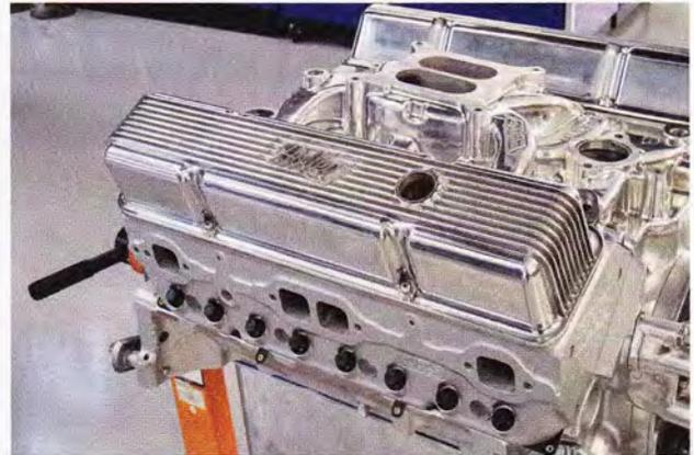
**24** Holley's new vintage-style aluminum valve covers fit all '58-'86 small-block Chevy engines with perimeter bolt patterns. Available finishes offered are as-cast, satin black with machined fins, and polished—valve covers are 3½ inches tall with pre-installed internal oil baffles (oil fill and PCV grommets also included).
