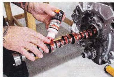
**04** Although roller cams eliminate some of the problems associated with breaking in flat-tappet cams, COMP Cams' installation lube is still required.
