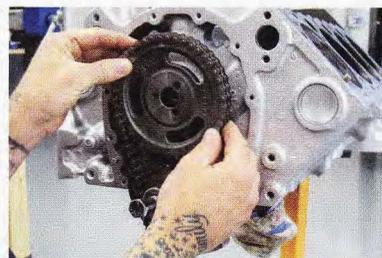
**05** To maintain accurate valve timing a COMP Cams roller chain and sprockets were installed straight up (neither advanced or retarded). Three keyways in the crank sprocket allow for 4 degrees of advance/retard.
