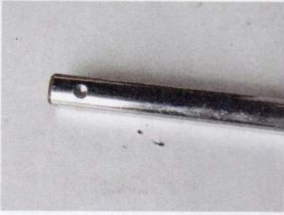
**15** Before the U-joints are attached, the ends of the shaft should be dimpled with a drill to provide a seat for the set screws.
