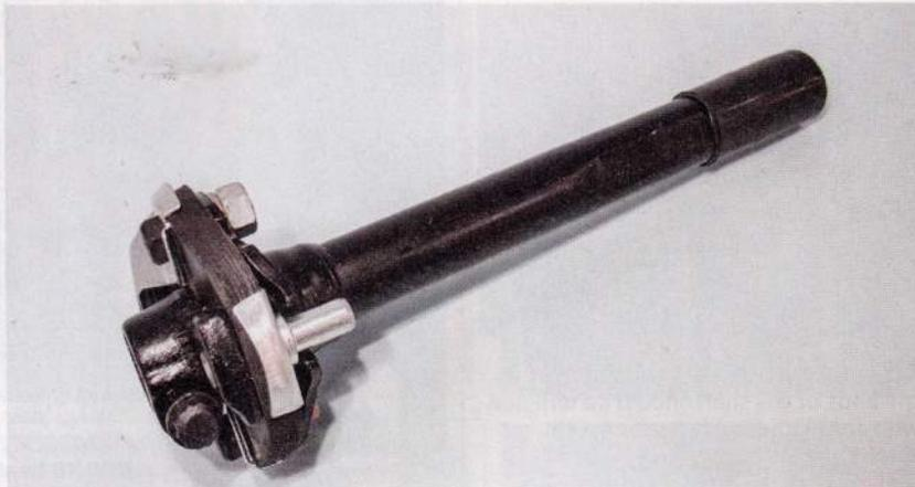
**17** For those wanting to retain the original intermediate shaft, or at least most of it, CPP offers this lower portion that allows the use of a 500 Series steering gear.
