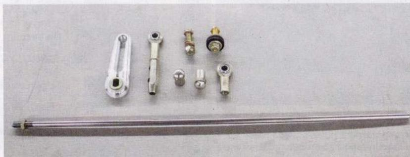
**18** One of the additional changes made necessary by the steering column sway is new shift linkage. Ours came from Kugel Komponenten.
