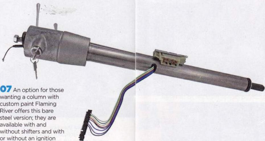
**07** An option for those wanting a column with custom paint Flaming River offers this bare steel version; they are available with and without shifters and with or without an ignition switch.
