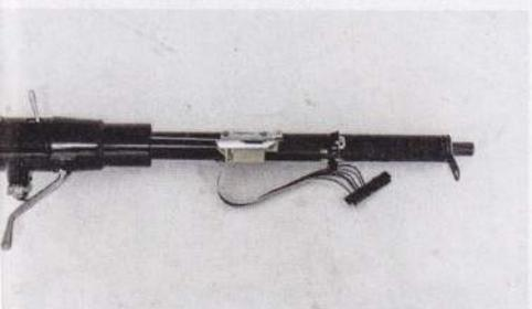
**06** As part of the steering upgrade we added a black, powdercoated tilt steering from Flaming River. Ours included a column shifter.
