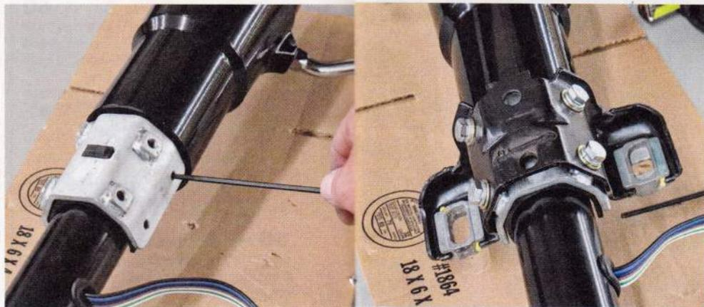
**09** The original C10 column-mounting bracket attaches to the Flaming River column.
