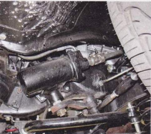
**04** Just like the original steering gear the CPP replacement bolts directly to the outside of the left framerail.
