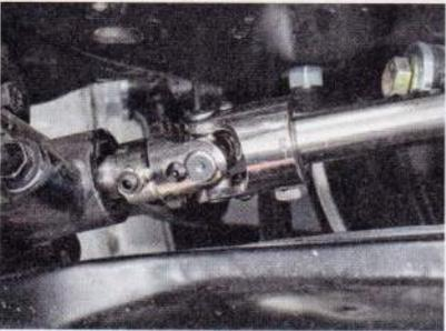
**16** The U-joints are secured with set screws with lock nuts. A thread-locking compound should be used on the fasteners and they should be checked after the first few miles.
