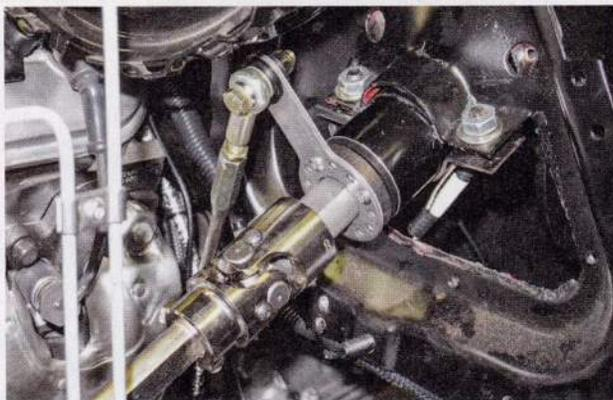
**20** Kugel's transmission arm is slotted to allow the travel of the column shifter to be matched to the gear positions in the transmission.
