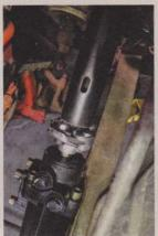
16 Taking into consideration the height of the rag joint (which has been removed here), the actual height we wanted the steering wheel (roughly 3 inches lower), the amount of steering shaft stick-out (2 inches), and between 1/2-3/4-inch gap between the column tube and joint gave us the numbers to start cutting and trimming.
