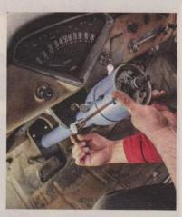
**32** Fully taped up to prevent any unnecessary marring or scratching, the 30-inch plain stainless column (TC-30-SB) bolts right up using the factory drop; because it's pre-fitted with a 1-inch DD inner steering shaft, it mates right up to the 400 box with the appropriate mini rag joint.
