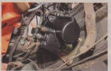
09-10 First, let's get the easy part out of the way - mounting the CPP 400 Series box. Using the provided Grade 8 hardware and bracket, simply bolt the box to the existing three holes in the framerail.
