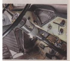
**33** And though it's not that complementary in its current condition, the stock '57 steering wheel bolts right on — with full operational horn facilitation.
