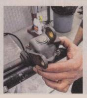
24-25 As with the original, the shortened column will get slotted to allow for finetuning adjustment of the shifter.
