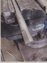
19 If your steering shaft is too worn, splines wasted, what have you, CPP offers replacement inner shafts as well (they too will require the rag joint modification).
