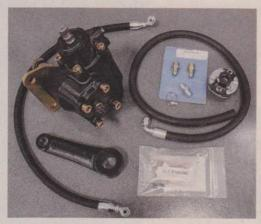
O2 You have choices, pertaining to steering column options, when using a 400 Series conversion kit: aftermarket (obviously), stock automatic, and stock manual. Best part about retaining a threeon-the-tree column you can also still retain the stock shift linkage mechanisms, as you'll
