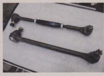
13 CPP offers both a stock replacement drag link (fixed) as well as a custom, adjustable one. In the unlikely event the OE steering linkage is slightly off, the adjustable link will fix that right up.
