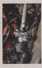
21 With a 2-inch stickout retained, the steering wheel was test fit to ensure the proper positioning and so too was the shift lever, which needs to be able to clear the dash during operation.
