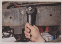
11 Now, using the new CPP Pitman arm (splines on the 400 box differ from OE, hence the reason we're not using the old Pitman), center the output shaft on the box.
