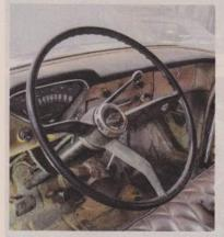
27 The linkage is once again bolted back onto the column and the shifter rod connector sleeve shortened accordingly — ensure full engagement of all gears is achieved before finalizing any shift linkage mods.
