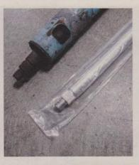
**20** The shaft and steering coupler should be a snug fit (not too loose where it's solely relying on the set screw, which you will need to drill a relief hole for once it's all set up).
