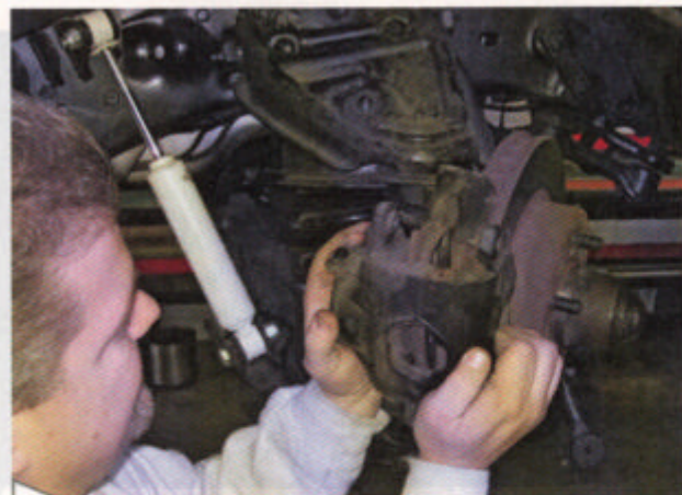
Let's make with the action. The '72 was equipped with the stock five-lug disc brakes, which is obviously a blessing compared to all the six-lug drum brake trucks out there. But all C-10 owners ('60-87) can benefit from what we're about to do. In order to get the new Modular spindle on, the brakes need to come off.
