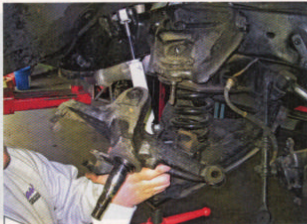
Most aftermarket dropped C-10 spindles like this one will only allow stock-type disc brakes, which is fine, but if you want to go to bigger brakes and wheels—like many do—than you'd have to buy another spindle. Not so with CPP's new Modular dropped spindles.
