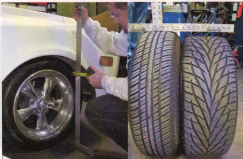
Before we started the install, we took some measurements of two sets of wheels on the '72 C-10 for reference: a set of 15-inch Cragars with tall/skinny 225/75R15 tires and a set of 18-inch Cragars wrapped in 255/45R18 Toyo Proxes S/T tires, which would be comparable with many larger-diameter/lower-profile tire combos found in the front.
