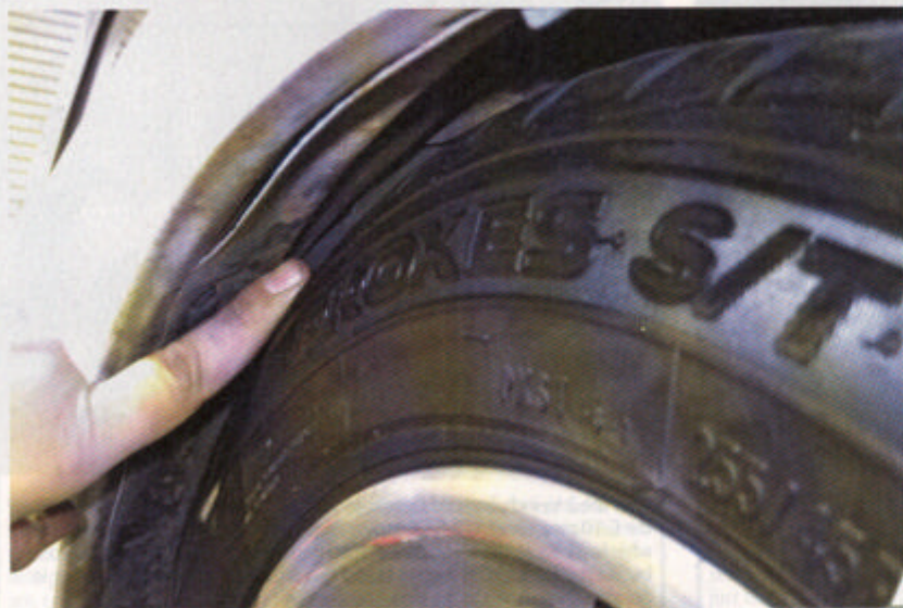
Before we started the install, we took some measurements of two sets of wheels on the '72 C-10 for reference: a set of 15-inch Cragars with tall/skinny 225/75R15 tires and a set of 18-inch Cragars wrapped in 255/45R18 Toyo Proxes S/T tires, which would be comparable with many larger-diameter/lower-profile tire combos found in the front.
