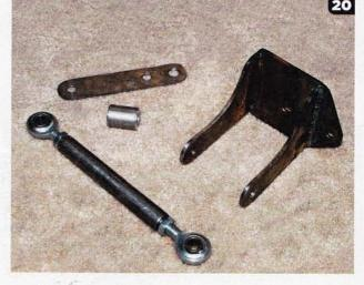
With the rod installed, I tried screwing it costs tighten the belt. It worked out pretty well too. In the next image you can see how everything mounts and lines up. The 1/2-inch rod is tapped for 3/8x24 left and right-hand Heim joints that allows you to screw it in and out for adjustment.
