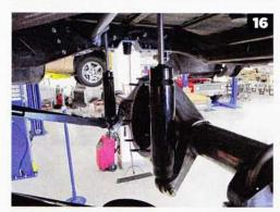
The CPP crossmember was slid into place and measured side to side and also front to rear to make sure it was square.
