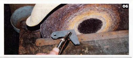
go and make some quick reference measurements. Using those I can come up with a pattern and then make the bracket. In this case I am going to use the area where the fuel pump usually mounts. This truck had an electric one so this worked out well. Adjustment will be with a threaded ½-inch steel rod with 3/8-inch male Heim joints. The Heims are left- and right-hand thread so you can adjust the belt by turning the bar. The bar attaches to the pump and then to a small bracket at the water pump.
