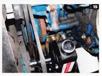
With the bracket bolted to the fuel pump boss and the pump bolted to the bracket, I can see my belt alignment is good and the bracket fits good as well.
