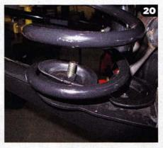
The springs can be attached and are held on by plates that go in between the spring. Shown are the upper and lower spring mounts.
