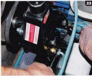
At this point all that was left was to install the hoses and fittings. The pressure side is the one next to the framerail and is always 16mm. The return side is 14mm on the 1979 and '80 boxes. These boxes have the straight splined input shafts - the return side on the 1980 to '85 boxes is 17mm and the input shaft is splined, but also has a groove machined in it for a lock bolt. By the way, Classic Performance Products can provide all the fittings you might need to complete the hose install.
