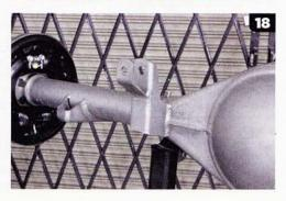
The CPP lower shock mounts were welded on the Currie rearend. Before welding I checked that the shock had clearance and that the shock didn't bottom out before the axle hit the bumpstop. CPP recommends that the shock not bottom out before full upward suspension travel.
