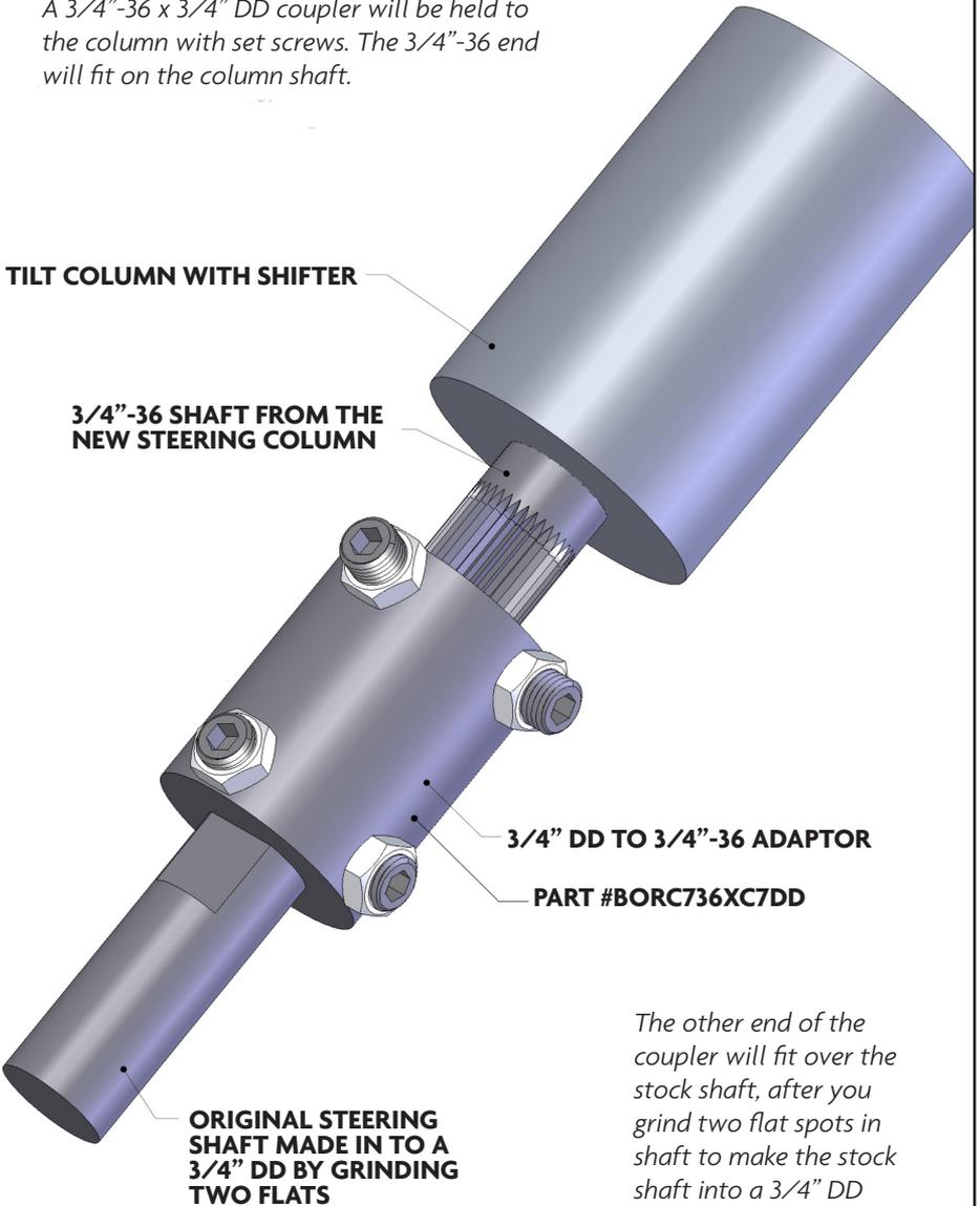
The other end of the coupler will fit over the stock shaft, after you grind two flat spots in shaft to make the stock shaft into a 3/4" DD shaft. (See "Synchronizing Your Column" on page 7.)
