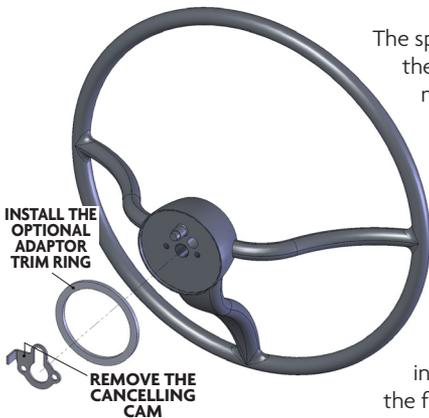
The spline in your stock steering wheel is the same as the one on the new column, so no modifications are needed here.
