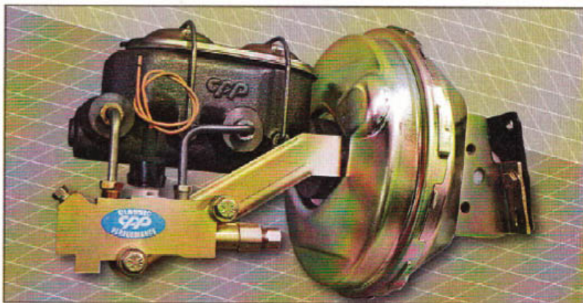
This combination of booster, master cylinder and proportioning valve is typical of what is found on most classic GM vehicles. While this set up was not an OE option until 1967, many vehicle owners today have upgraded to this safer style of braking. A company like CPP (which sells this particular unit) has them available in all sorts of sizes and finishes from plain to chrome and polished aluminum.
