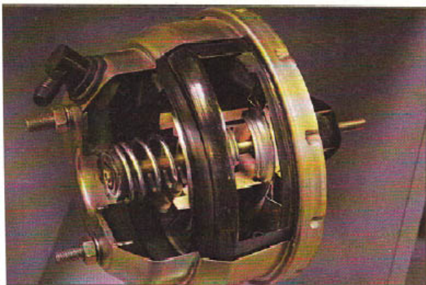
Externally brake boosters look no more complex than a soda pop can, internally it is a different story. Take a look inside this cut away dual diaphragm booster. Booster rebuilding is not a do it yourself type of job.
