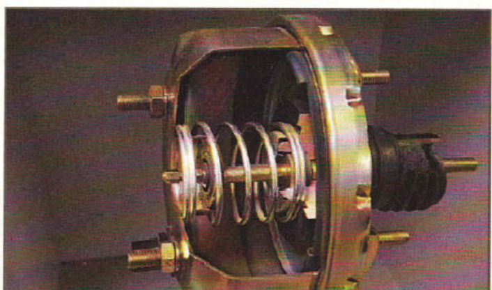
Now take a look inside this single-diaphragm booster. It may appear less complex than the larger dual diaphragm booster, but it functions in exactly the same manner. Opening up a booster can have adverse effects on its future functionality, so resist the urge and keep them closed.
