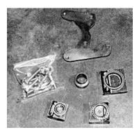
The Classic Performance Products disc brake conversion kit includes new bearings and bearing cups, two caliper brackets and all necessary mounting hardware.
