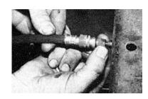
19. Attach the other end of the rubber brake hose to the hard line the same way as you removed the stock version.
