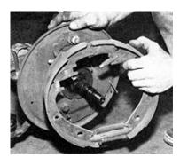
3. After removing the return spring, the entire brake pad assembly can be taken off.
