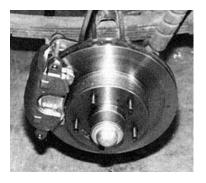
21. And there you have it! Disc brakes on a straight axle classic with no major modifications. Remember that you must decide whether you are going to upgrade to power brakes, or stick with the manual setup. There are a host of power brake options that are determined by application.
