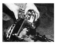
16. To install the caliper, the piston side faces inboard and the pressure relief nut faces upward.
