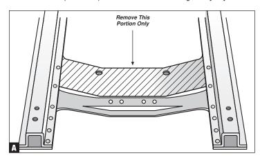
We find it the easiest to have the front sheetmetal off the car and starting with a bare front 'rail setup with all stock suspension removed. This provides the most amount of space to work with.
