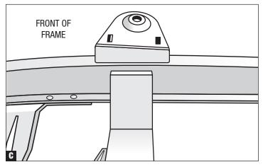
car more stable at highway speeds. With positive caster, the upper ball joint will be rearward of the lower ball joint. This is a very important step to ensure these are installed correctly. Tack weld these in place when you have them perfectly square to the lower crossmember and again making sure the angle is tilted back. (Fig. C)
