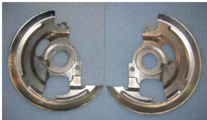
Photo 3: Shows a complete left and right set of dust shields modified to clear the lower arms.
