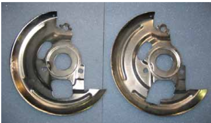
Photo 2: Shows drivers side dust shield. The one on the right has been modified to clear the lower arm.
