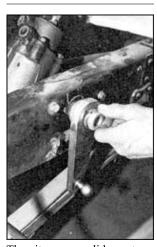
The pitman arm slides onto the output shaft and is torqued to 110 ft-lb. But first we made sure it was centered by rotating the shaft as far as it would go in both directions and splitting the difference.
