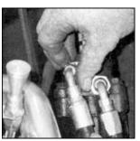
Alan threaded both the pressure and return hoses into place and routed the return hose over to the pump.
