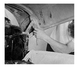
There's no welding necessary—all you have to do is drill a few holes. We picked up a kit from Classic Performance Products and installed it in just a couple of hours. Follow along as we install a stainless steel reverse-tilt hood kit on a '56 Ford F-100. The common saying is that the original Ford hood opening system didn't work all that well when hey were new (46 years ago For a '53 Ford). While a friend supports the hood, take off
