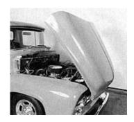
If you've got an engine compartment worth showing off, a reverse-rilt hood is a visual eyepopper.
