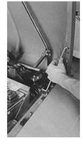
Now you won't have to worry about the wind blowing your hood shut. This prop rod stays out of the way so that you can work on your engine.
