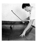
Unbolt the support rods and then wiggle them back and forth to loosen the plug-welded areas. The paint will usually crack and reveal the welds.
