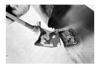
Drill out the welds ta removethe support rods. Be careful not to let the in too far. Using a depth gauge as a socket or two slipped over the drill) will help prevent damage.
