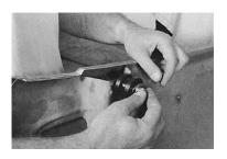
These slick Teflon rollers bolt right up to the existing hole. A nut is to the inside for extra security.
