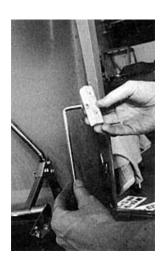
This nice piece is attached to the hood to give the prop rod something to attach to.
