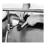
A small portion of the metal lip on the underside of the hood will need to be trimmed. After the framework is positioned, mark the area.
