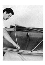
After bolting the underhood framework together, bolt it to the existing holes with the supplied hardware.
