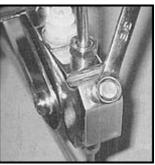
On the proportioning valve, the right front line was plugged off. Instead of running this additional line, the left front line will go to a "T" fitting located inside the framerail. From the "T" fitting, the front lines then split off and go to the front left and right wheels.
