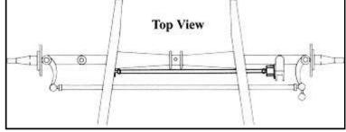
Though designed for use with TCI frames and suspension parts, the front panard rod can be adapted to most any chassis using a 4-link, transverse spring and a beam or tube axle.
