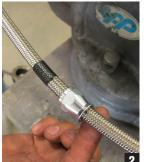
2. Slip female collar fitting onto the stainless line before cutting (threads pointed toward end to be cut), as it may want to fray freshly cut wire braid if done afterward. (Fig 2)
