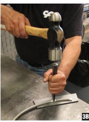
3. There are a few different methods in which to cut the braided stainless: preferably is by using a high-speed, thin-bladed cutoff wheel (Fig 3A); however, an extremely sharp chisel and heavy hammer also work well (Fig 3B), but care needs to be taken to "not" pinch the inner Teflon tube (a similar-sized punch can be used to reshape the Teflon after it's been cut).
