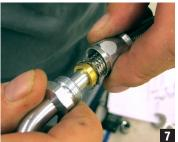
7. Before completing your fitting by fully tightening, mock up in the vehicle and position the fitting angle—mark with a Sharpie to help keep positioned. (Fig 8)
