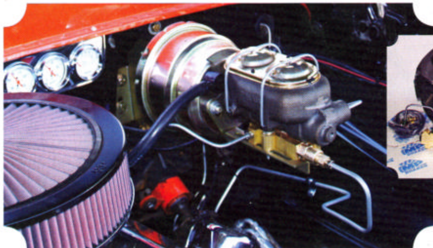
■ Above: Master Power Brakes's DB1545P Power Front Disc Brake Kit for 1965-1972 Ford half-ton, two-wheel drive pickup trucks with twin I-beam suspension comes fully assembled. ■ Left: The kit shown installed.
