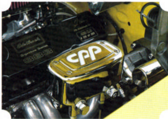
■ CPP's MCPV-1 combines the master cylinder, double adjustable proportioning valve, removable metering valve and stop light control in one lightweight unit.
