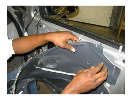
Remove plastic environmental barrier from door frame and discard.
