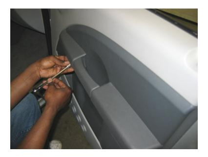
Remove door panel from door disconnect all hardware and wire harnesses between panel and door.
