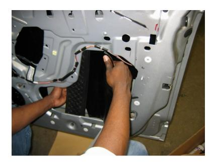
Position the sheet against the outer skin by using the smaller access holes through door frame. Cover a minimum of 70% of the door skin starting in the center and work toward the outer edges of the door.
