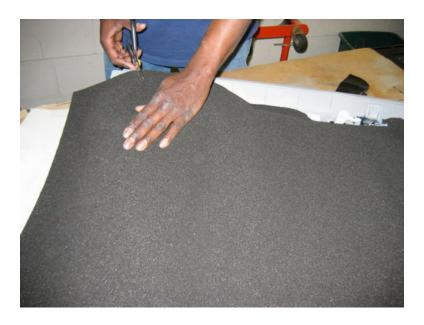
Cut away any foam that overhangs the edges of the door panel with scissors or a utility knife. Hand press the foam to the panel across the surface.
