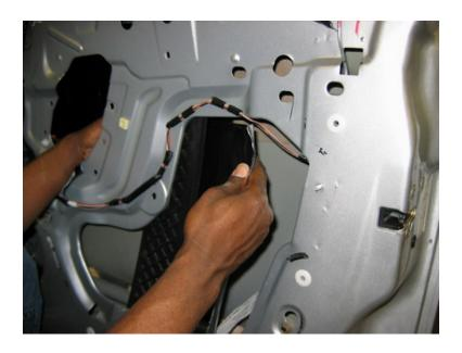
Apply HushMat Ultra Silver or Black Foil damping material to the inside of the outer door skin by removing the brown release paper from the Ultra and passing the sheet through the largest access hole in the frame. Several installers prefer HushMat Ultra black foil as it does not reflect light and will not be seen through speaker grills and other holes in your door.
