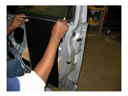
For the highest performance we recommend taking the larger sheets of HushMat Ultra and apply them to the door frame covering all access holes through the door. Start on one edge of the door frame and peel back the brown release paper from the sheet and apply from the top of the frame to the bottom. The HushMat Ultra also serves as the vapor barrier that you removed.
