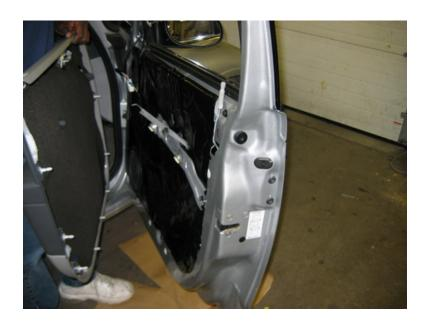
Secure all hardware and electrical connections from the door panel to the door and place the panel back onto the vehicle. Test each device to ensure function before securing the panel.
