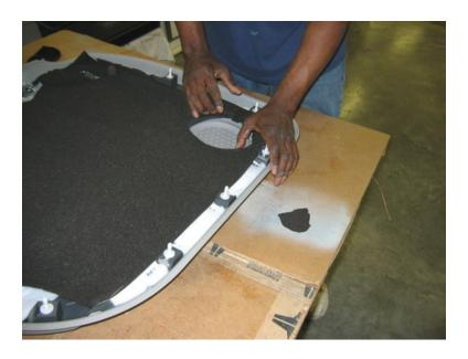
Cut around all panel fastening points, speaker grill, wire harness pass through of any mechanical hardware the will be attached to the vehicle door by slitting the foam and pulling the device through the foam.
