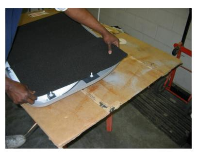
Lay the door panel on a table with the back of the panel facing up. Lay one sheet of Silencer Megabond 1/4" foam against the door panel with the white release paper on the foam. Place the edge of the foam just inside the fasteners or clips that secure the panel to the door.
