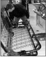
13..However, before lighting the torch to begin welding, you'll want to check the seating position and the brake pedal position.
