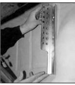
6.. The trimmed mounting bracket was held in place to check the length, and to see where it might be positioned against the firewall.
