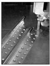
5..Both mounting brackets were cut to the same length. The rows of holes are for the master cylinder and booster mounting bracket. They should be 90 degrees from the firewall. The brackets also have mounting holes if you decide to bolt the assembly to the firewall.
