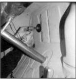
17..Since this unit will be welded in place, you'll need to remove the primer on the firewall for a stronger and cleaner weld.
