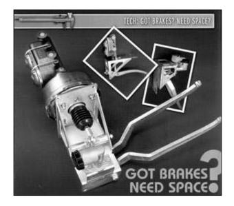
Classic Performance Products makes it easy to steer your Install a 90-degree under-dash swing pedal and master cylinder assembly.
