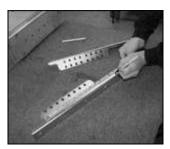
3..Then mark a 13-inch section of the bracket and trim both ends on the band saw.
