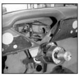
11..This is the optimum position that CPP feels will allow the driver to be comfortable and allow the bracket to mount securely to the firewall.
