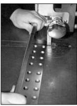
4..The band saw makes quick work of cutting the mounting brackets to the exact length for this installation. A rotary cutoff tool will also get the job done. Or you can make your own mounting brackets from angle iron and save a
