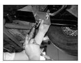
Four holes needed to be drilled in the trailing arms and then the mounts were installed using the supplied hardware.
