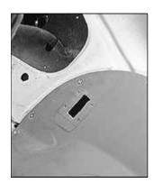
The pedal mounting base can then be bolted in place. The same fasteners also hold the cable bracket in place under the floor.
