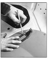
Using the cable bracket as a template (locating it 3/4-inch up from the bottom of the pedal), Alan marked the floor where it needed to be drilled and cut.
