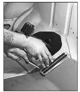
Finding a proper mounting position is probably the most critical part of the installation. Your best bet is to sit in the driver's seat and find a spot that will be comfortable for long-term driving. You'll also want to check under the floor to make sure there aren't any obstructions. Once you've found the spot, lay the pedal flat on the floor and mark its position.
