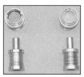
The TV boost valve and reverse boost valve were replaced with larger bore components as shown on the left. This increases internal trans pressure and clamping force across the board.
