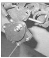
Last, but certainly not least, we installed the TV Made EZ system from Bowtie Overdrives. The key to their success is this cam mechanism that is made specifically to work with the linkage of all the popular carburetors. Combined with the carb base plate Bowtie Overdrives supplies, it eliminates much of the guesswork associated with TV cable adjustments.
