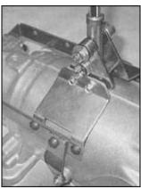
Before installing the 700-R4, the Gennie Shiffer base brackets were bolted into place on the trans.
