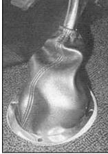
The finishing touch before the test drive was dropping the shift boot over the shifter. Here it's awaiting the four screws that secure the bezel to the floor.
