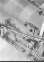
We also set-up the shift linkage at this time. It's recommended that you set it up with the trans and shifter in drive and then check the other gears.
