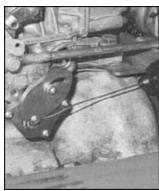
The cable was secured at the trans, and the base plate bracket was installed under the carb. The cable was snapped into the bracket and linkage adapter, and then the cable length was set by depressing the lock on the cable and opening the throttle fully. Then the cam can be adjusted to fine-tune the timing and firmness of the shifts and downshifts.
