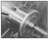
At Phoenix Transmission Products, every drum is machined across the band surface to ensure a perfectly flat and concentric surface for band application. If it's not flat, the band will only clamp on the high points causing slippage.
