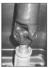
Inland Empire Driveline took just over 5 inches out of the driveshafl so we could reinstall it with the 700-R4. Check elsewhere in this issue for some driveshafl tips.
