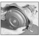
We filled the converter with as much fluid as we could without it spilling out and installed it onto the input shaft.
