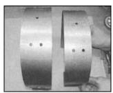
A stock band (right) is not as wide and does not cover the full drum surface. The Phoenix replacement band (left) is wider and covers the full area of the drum surface. This is important because with more band surface contacting the drum, less slippage occurs. It's like adding bigger brakes to a high-performance vehide. The band anchor area is both reinforced and hardened to prevent fluctuations in adjustment over time.
