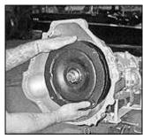
1..First things first don't forget to install the torque converter! I know it's a simple step, but I have the attention span of a gnat. And before that, top it off with fluid. Slide the converter onto the tranny while turning it back and forth to seat it all the way into place.
