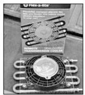
20..Now we needed a way to keep the tranny cool. We opted for this Flex-a-lite unit (PN 4190) with its own electric fan so it can be stuck somewhere out of the wind and still work.
