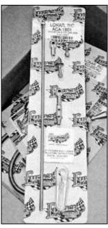
11..But first, we need to be able to grab the gears! CPP provides the means to hook just about anything up to whatever you might need, and they had just the ticket to connect the C-4 to the shift linkage on the ididit steering column.
