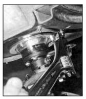
16..A slight counterclockwise tweak with a big adjustable wrench on the shift lever off the column made things line up much better. Now the rod end at the column isn't maxed out.
