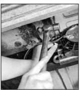
22..We chose a spot out of the way of exhaust, plumbing, and road debris, which wound up being on the outside of the passenger side framerail just behind the doorsill. Using a transfer punch makes marking the holes much easier and eliminates curse words.
