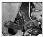
10. The firewall hole was widened slightly to allow full motion for the linkage.
