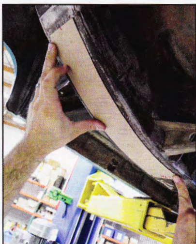
9. A pattern was made of the pocket mount, which was then transferred onto the underside of the chassis rail.
