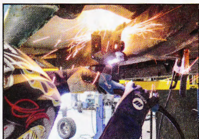
6. The spring hanger brackets were removed from the frame rails using a Miller Electric Manufacturing Company plasma cutter.
