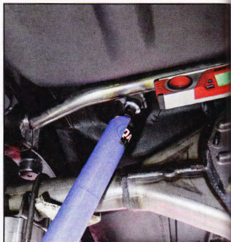
29. Located perpendicular to chassis and perfectly horizontal in relation to the chassis, the crossmember is ready to be welded. Note the rearend is as high as it can go (bumpstops will actually stop it going this high) to ensure the shocks don't bottom out before the suspension reaches full compression.
