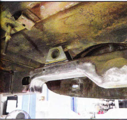
19. The notch plates and spring shackle mounts were then fully welded.
