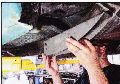
7. Mocking up the location of the front spring pocket mount. The bolt hole in the pocket must be centered in the frame access hole.
