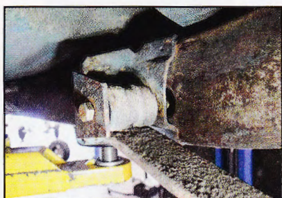
4. Disassembling the front spring mount is as simple as removing the bolt from the bush in the spring eye.
