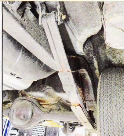
2. The stock leaf spring and hangers locate outside the frame rails, limiting the width of tire usable.
