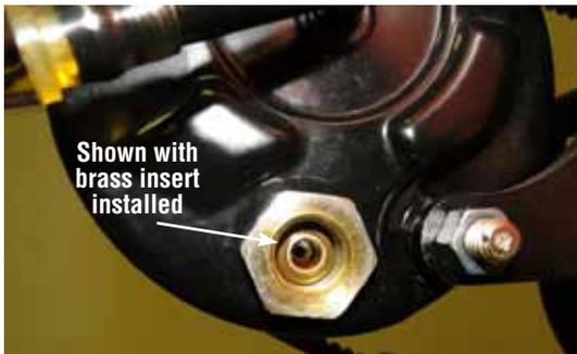
Be sure to use a line wrench to tightening down all fittings. Install the hoses into the rack. Tighten them down snug. **Do not over tighten.**
