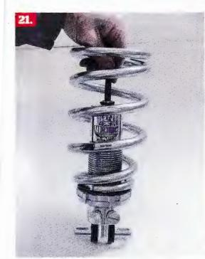
21. Along with spring preload adjustments, the two knobs on the shocks provide compression and rebound tuning. For this application, 500-pound springs were installed.
