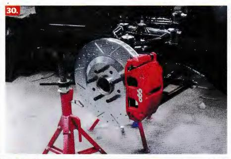
**30.** To provide braking power on par with the improved handling, CPP offers a variety of brake kits. This is their 13-inch Twin Piston Caliper kit that comes with the CS spindles; it's recommended for 16-inch or larger wheels.
