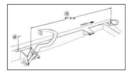
The Model 'A' brake pedal-master cylinder assembly is positioned as follows:
