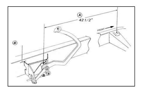
The '32 Ford brake pedal assembly is positioned as follows:
