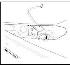
Mounting the '42-'48 Ford brake pedal assembly requires some minor cutting and redrilling. Using the template provided on the back of this sheet, and the instructions below, the pedal assembly is easily installed.
