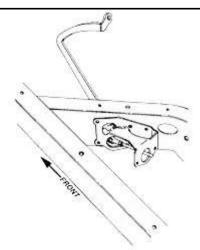
Mounting the '33-'34 Ford brake pedal assembly requires some minor cutting and redrilling. Using the template provided on the back of this sheet, and the instructions below, the pedal assembly is easily installed.
