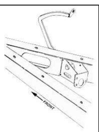
Mounting the '35-'40 Ford brake pedal assembly requires some minor cutting and redrilling. Using the template provided on the back of this sheet, and the instructions below, the pedal assembly is easily installed.
